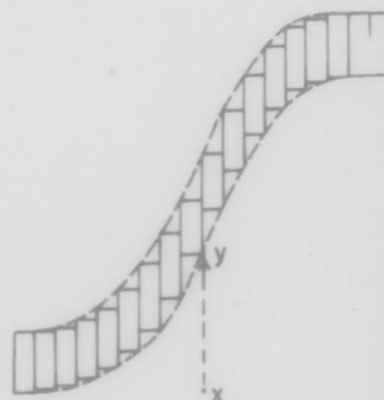
d. Similar folding with thinning of limb accomplished by cleavage folding (vertical shear cleavage).
