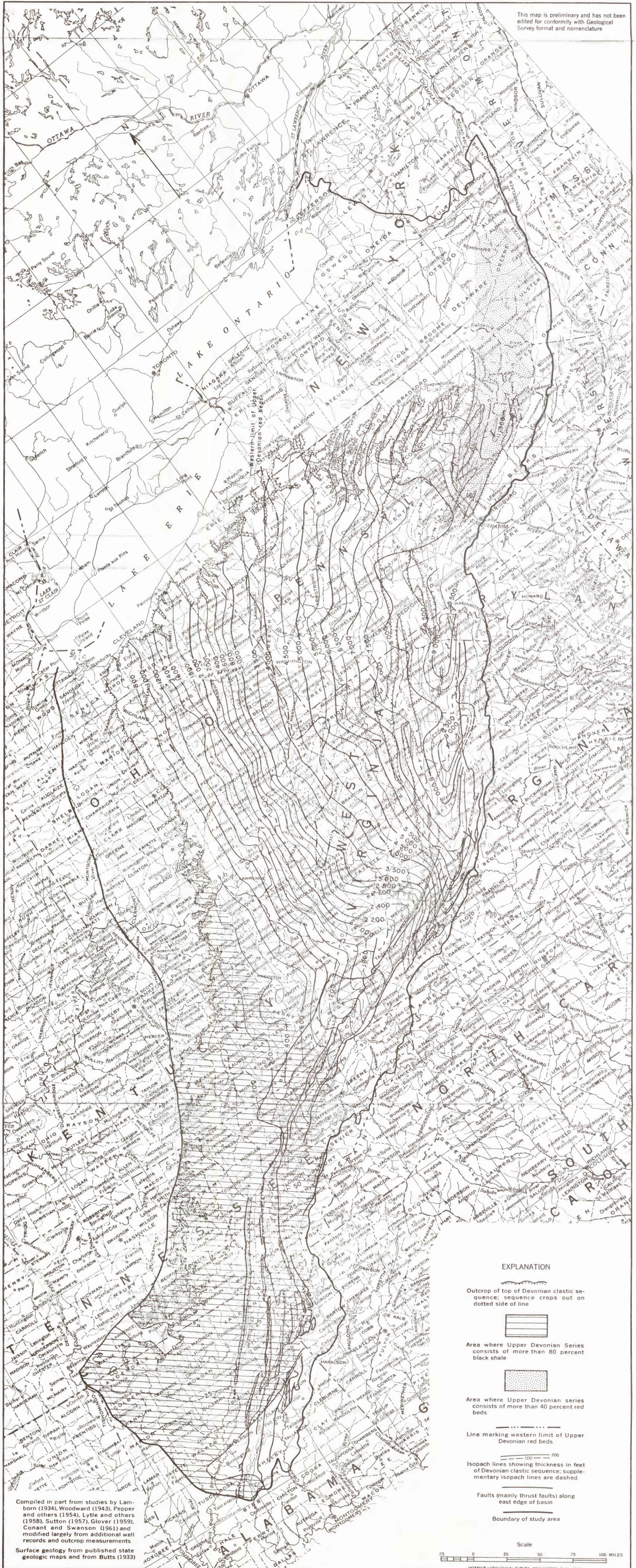
FIGURE 15.—MAP SHOWING SURFACE GEOLOGY AND THICKNESS OF THE DEVONIAN CLASTIC SEQUENCE, AND DISTRIBUTION OF SOME ROCK TYPES
