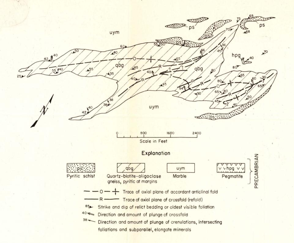
Figure 8. Inferred form of the peripherally pyritic, quartz-biotite-feldspar gneiss in the Fullerville-Edwards marble. This interpretation is based largely upon the geologic features shown on plate 1 together with petrographic studies of the rock layers.
