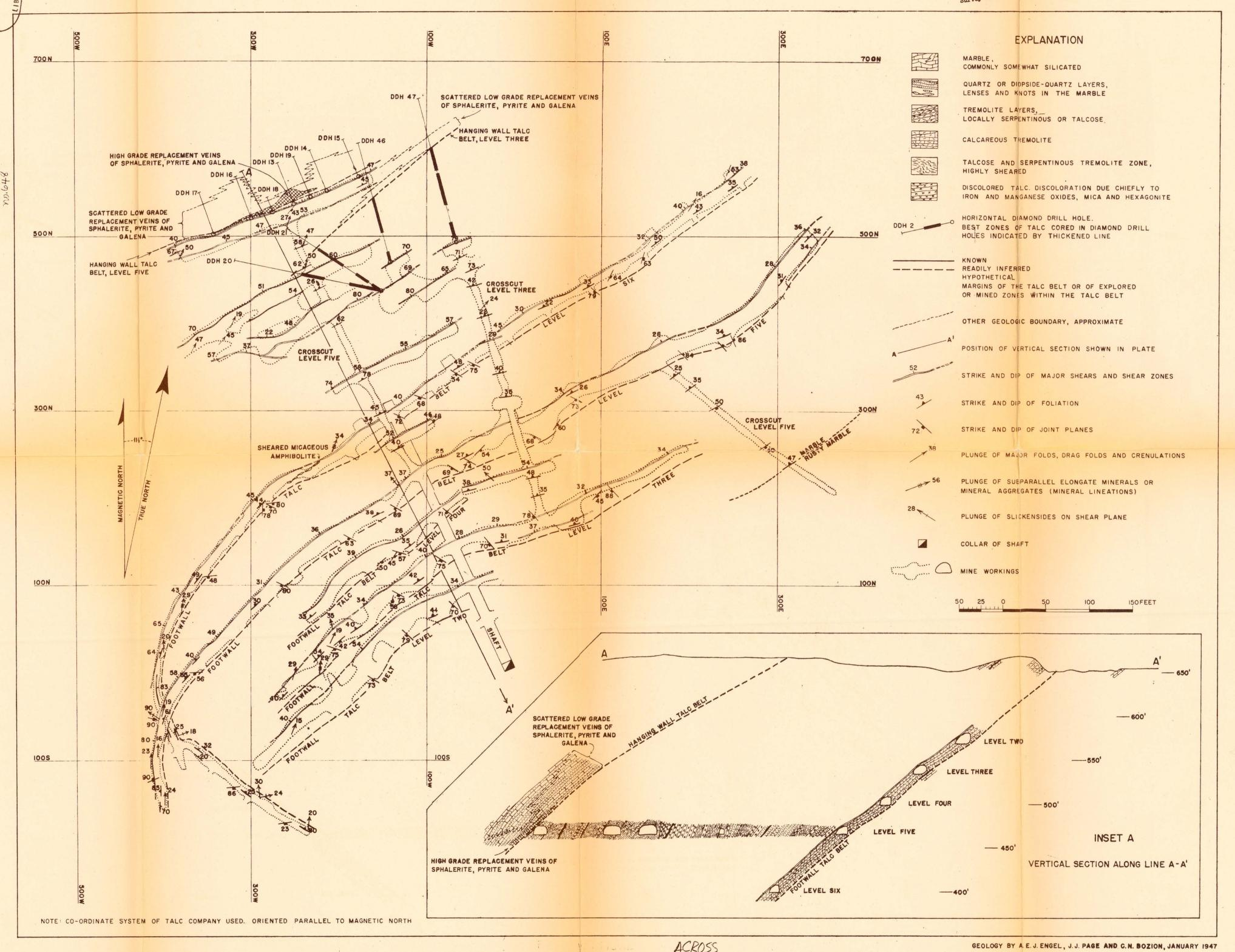
SUBSURFACE GEOLOGY AND SECTION OF THE WIGHT MINE
