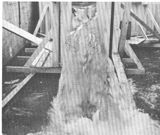
D. Upstream view of Run C-1 Discharge 21.5 cfs
