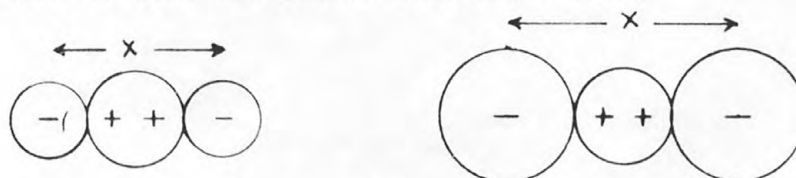
f. paired monovalent sites at the minimum separation about a divalent cation (as r^- increases, x increases)
