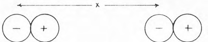
d. monovalent cations and paired monovalent sites with site separation x (position of lowest energy)
