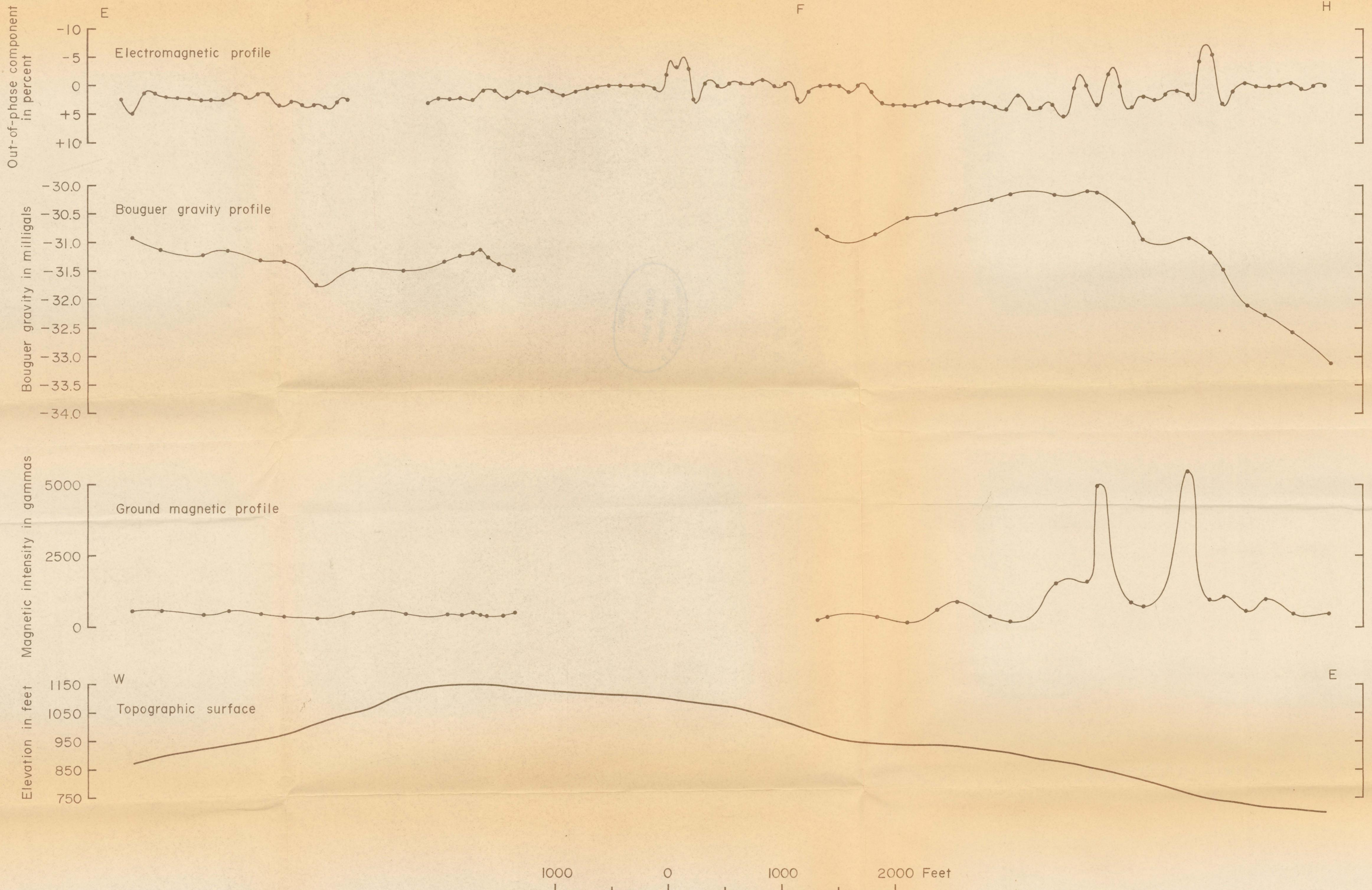
FIGURE 5. --Electromagnetic, Bouguer gravity and vertical intensity ground magnetic profiles along traverse E-F-H.
