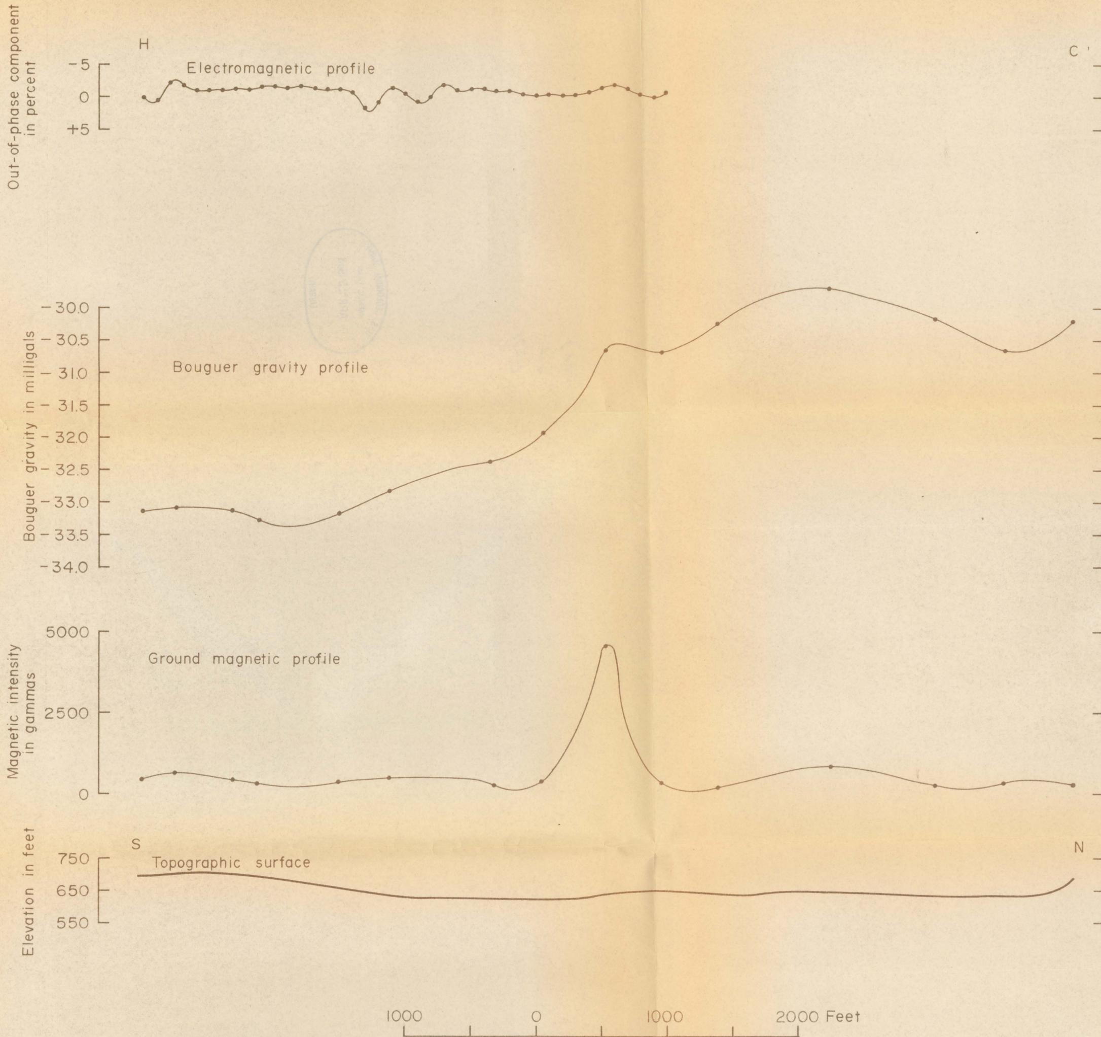
FIGURE 4. --Electromagnetic, Bouguer gravity, and vertical intensity ground magnetic profiles along traverse H-C'.
