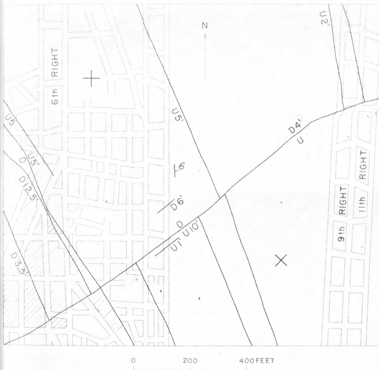
Figure 7.--Map of a part of the right side of the Sunnyside No. 2 mine showing the extensive damage center (+) and the seismic location (x) of a very large bump which occurred at 7:50 a.m., Dec. 24, 1963. Pillars that have been extracted are indicated by crosshatching.
