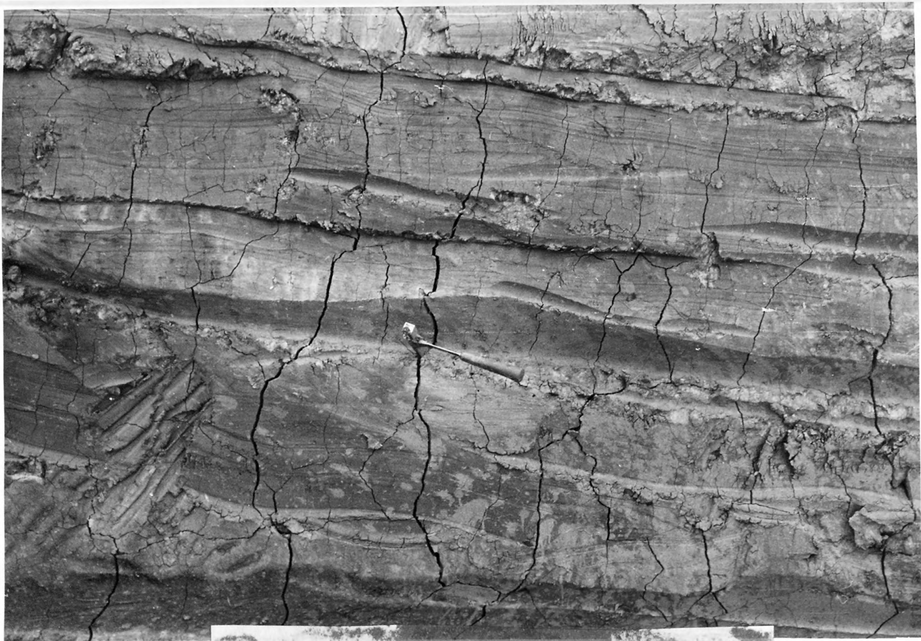
Figure 3. East wall of the excavation of Greenbelt, Maryland, showing the joint set in the clays of the Patapsco Formation of Cretaceous age. (Photo by author)
