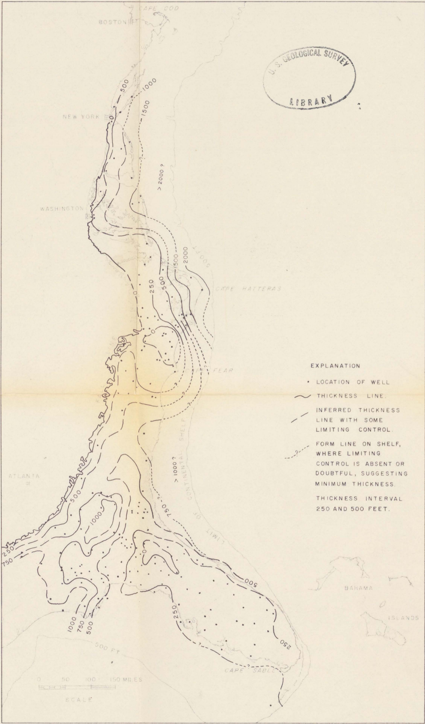
PL.19 THICKNESS OF ROCKS OF WOODBINE AND EAGLE FORD AGE ALONG THE ATLANTIC COAST
