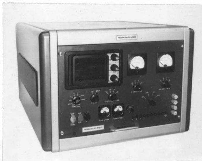
Figure 14. Prototype line-discriminator showing the optical unit and the control console (courtesy of the Perkin-Elmer Corp.)
