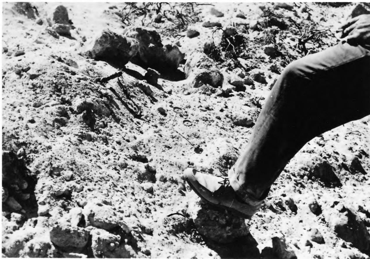
Figure 5. Photograph showing thermometers placed in ejecta of near west rim of crater 38. Note shadows cast by large fragments.
