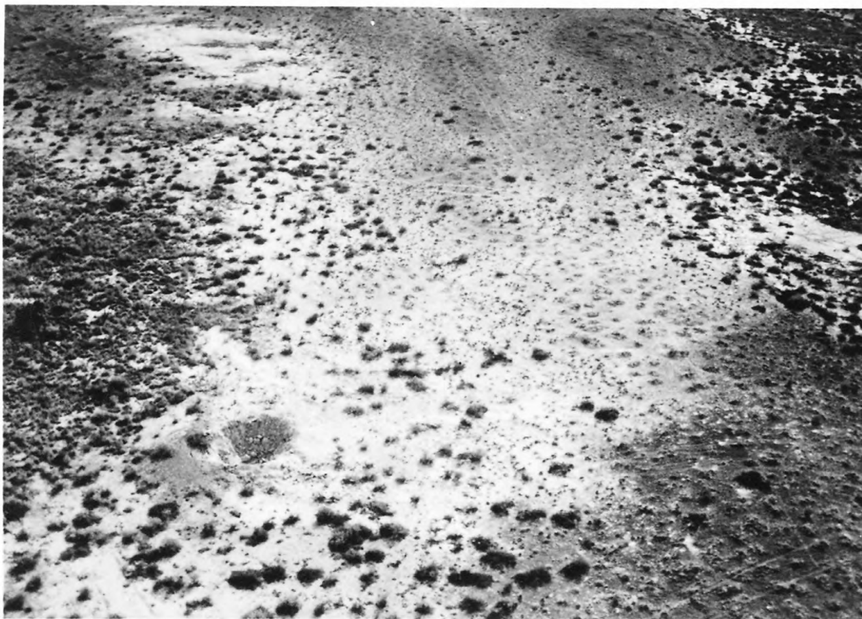
Figure 7. Photograph showing crater 38, ejecta, and fallout. Note fixed dune to right and large variations of reflectance of surroundings.
