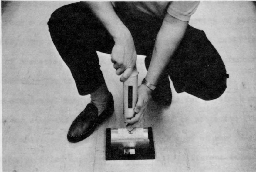
Figure 4.--Method of using the L-type Schmidt hammer and core holder.
