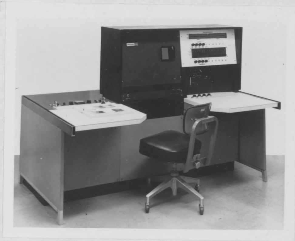
Figure 1.--Console for electronic image enhancement system. Right, electronic image processor; center, color video display; left, light table and master power panel.
