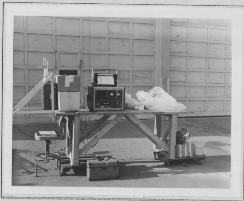
Figure 2. FLD mounted on casters for ground test over fluorescent granules, Menlo Park, Calif.
