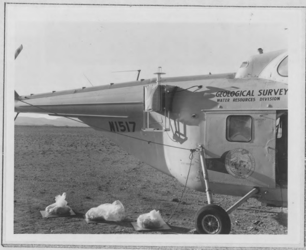
Figure 1. FLD mounted on H-19 helicopter during tests of response to fluorescent granules, Needles, Calif.
