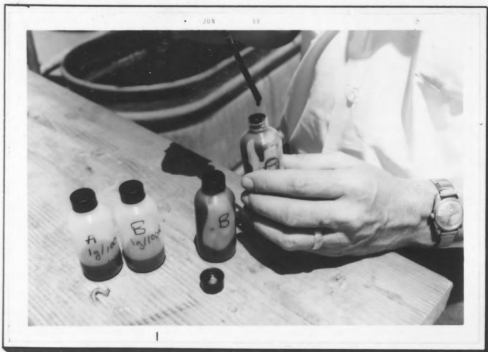
Figure 3. Crude oil from the Santa Barbara offshore leak, used in FLD tests (May 28, 1969, Menlo Park, California)
