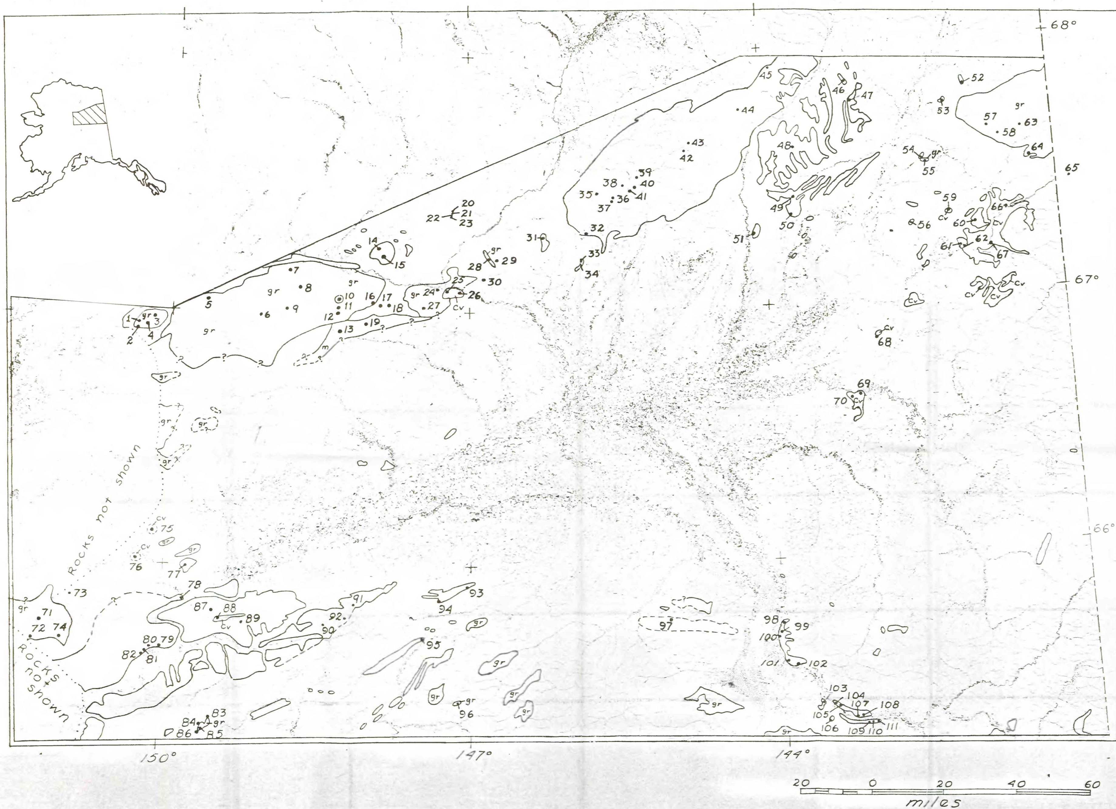
Fig. 1. Yukon River - Porcupine River area, showing location of magnetic susceptibility samples (by map number), and outcrops of granitic rocks (gr), Cenozoic volcanic rocks (Cv), and older mafic and ultramafic rocks (unlabelled outlines).
