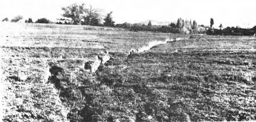
Figure 4.--Fracture along Bartın River east of Bartın, developed by slumping and landspreading.
