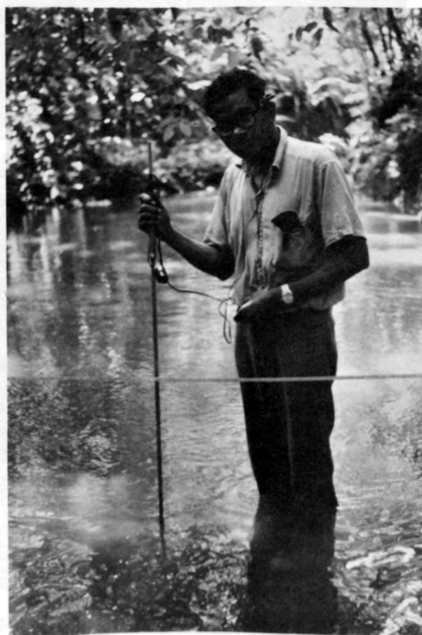
Figure 4. Measuring small stream on Dublon Island, Truk Islands.
