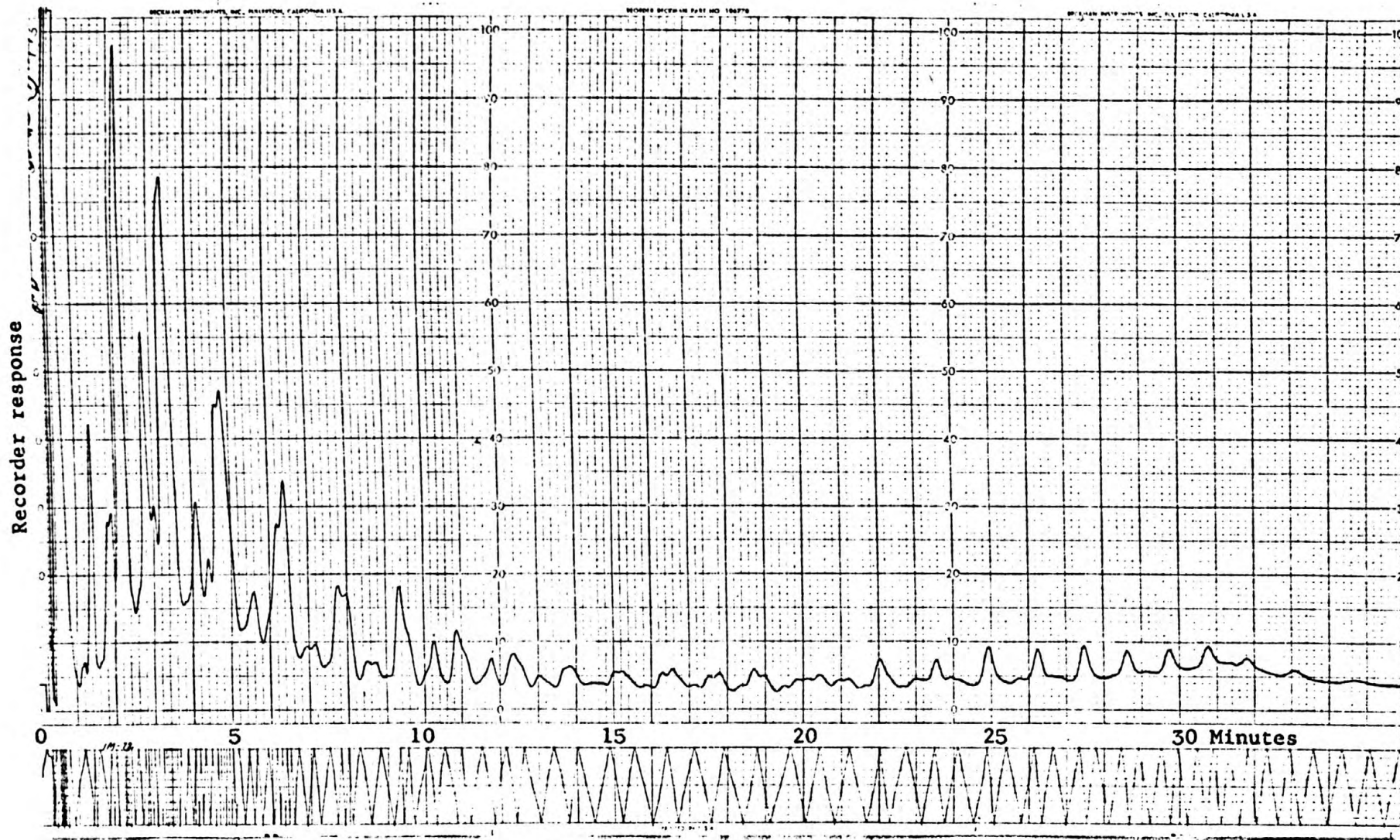
Figure 12. - Gas chromatogram of Andys Mesa oil, branched-cyclic saturated hydrocarbon fraction
