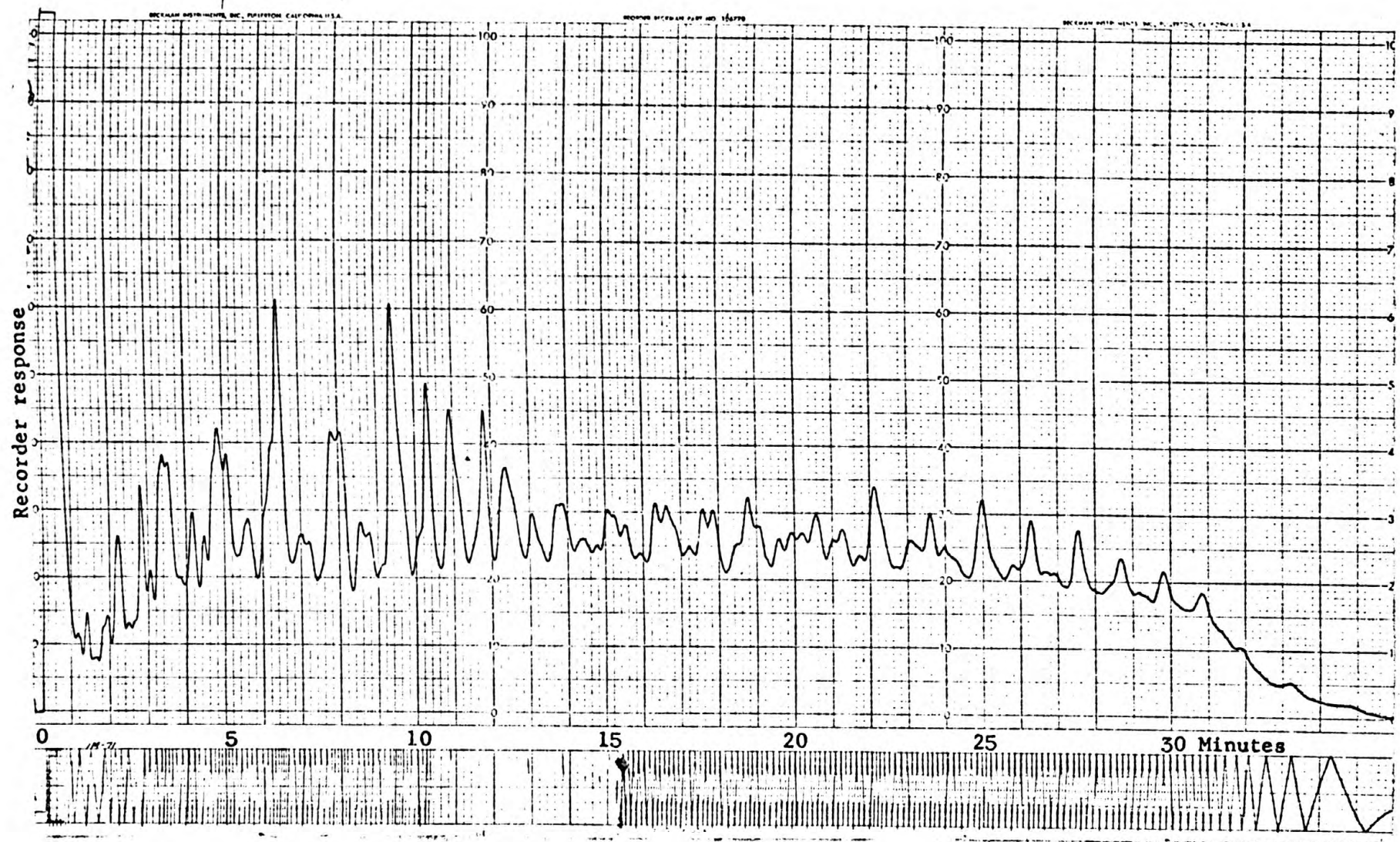
Figure 13. - Gas chromatogram of Papoose Cañon oil, branched-cyclic saturated hydrocarbon fraction
