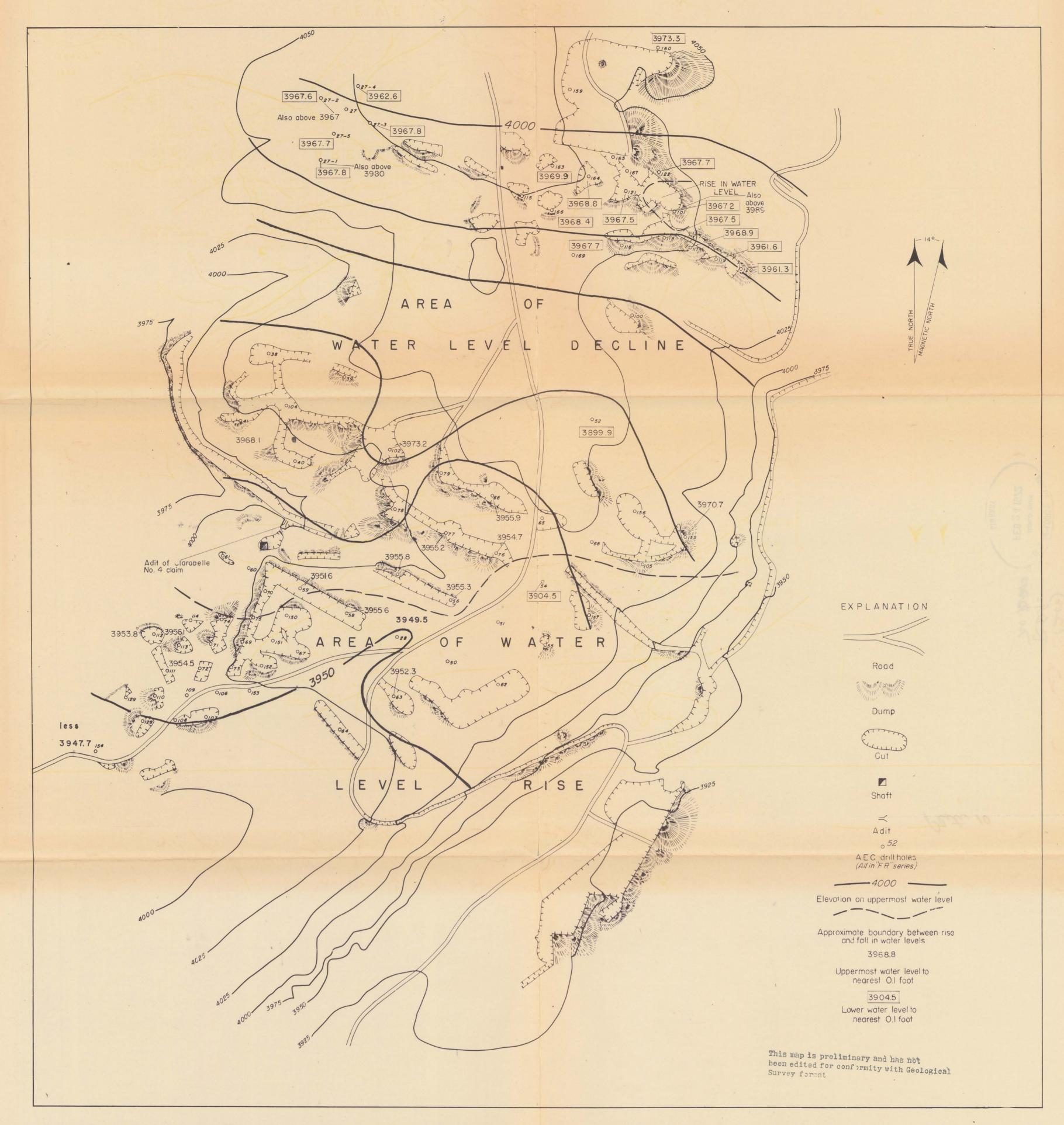
FIGURE - MAP SHOWING CONTOURS ON THE UPPERMOST PERCHED WATER TABLE ON AUGUST 7, 1954 IN PART OF THE CLARABELLE CLAIMS 1, 2, 3, AND 4, FALL RIVER COUNTY, SOUTH DAKOTA
