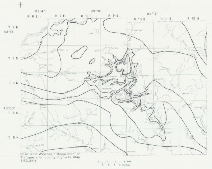
Figure 9. Saturated thickness of the sandstone aquifer.
