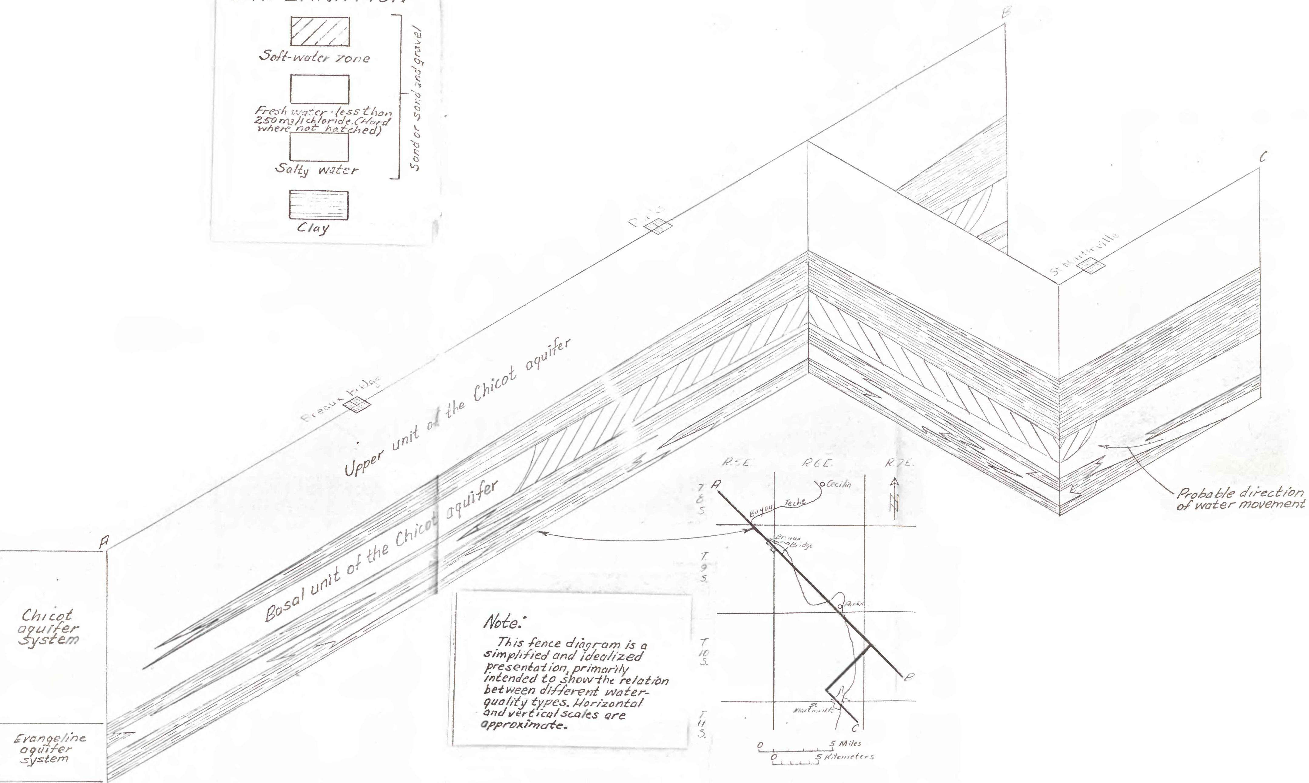
Figure 5. Diagrammatic section showing generalized geohydrology of the Bayou Teche area
