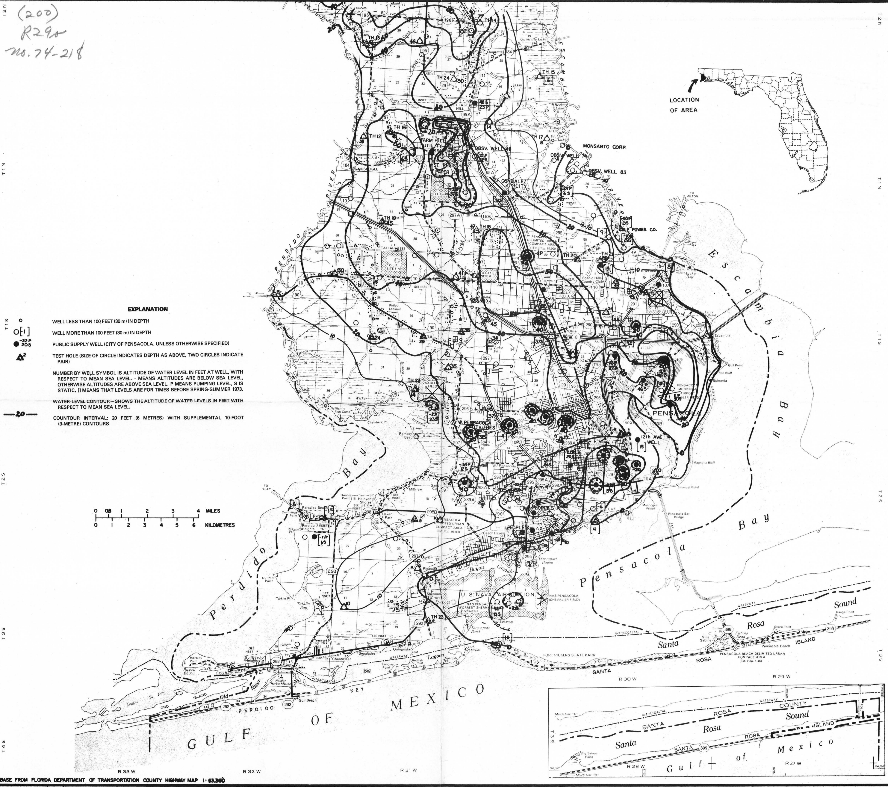
Figure 7.—Map showing approximate altitude of water levels in sand-and-gravel aquifer wells 100-300 feet (30 to 91 metres) in depth, Spring-Summer, 1973.
