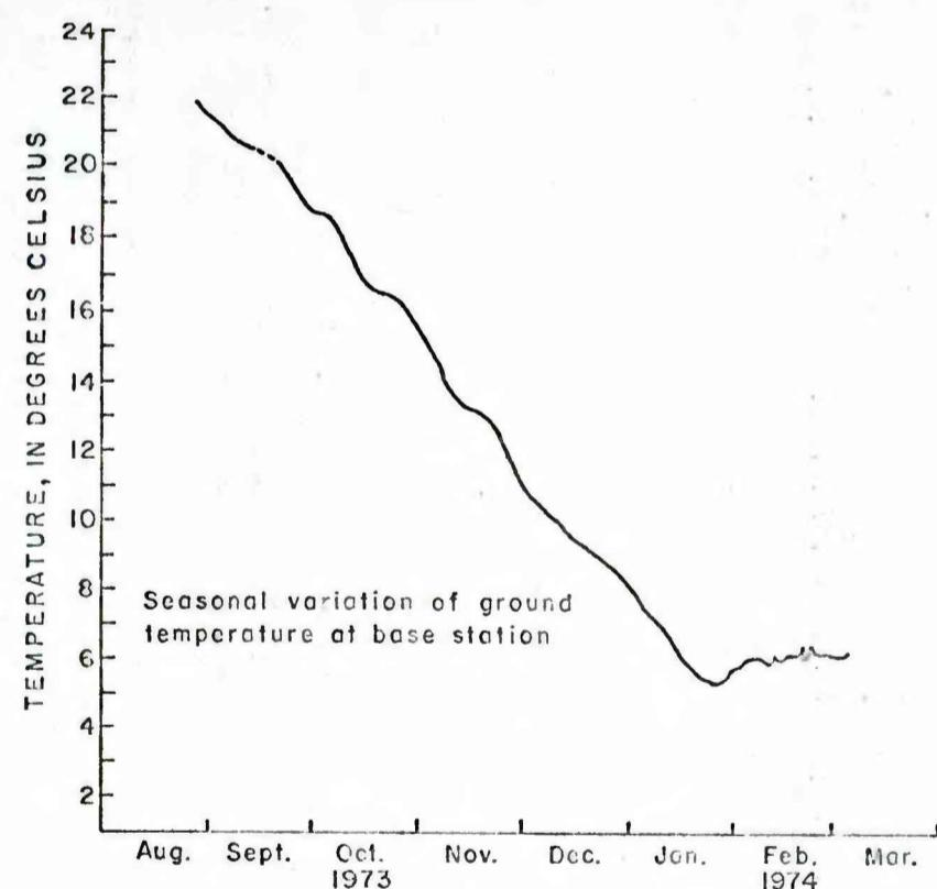
FIGURE 7.--Lines of equal ground temperatures, extrapolated and adjusted ground temperature at measuring sites, and the seasonal variation of ground temperature at 1-metre depth in the Weiser Hot Springs subarea, Idaho.
