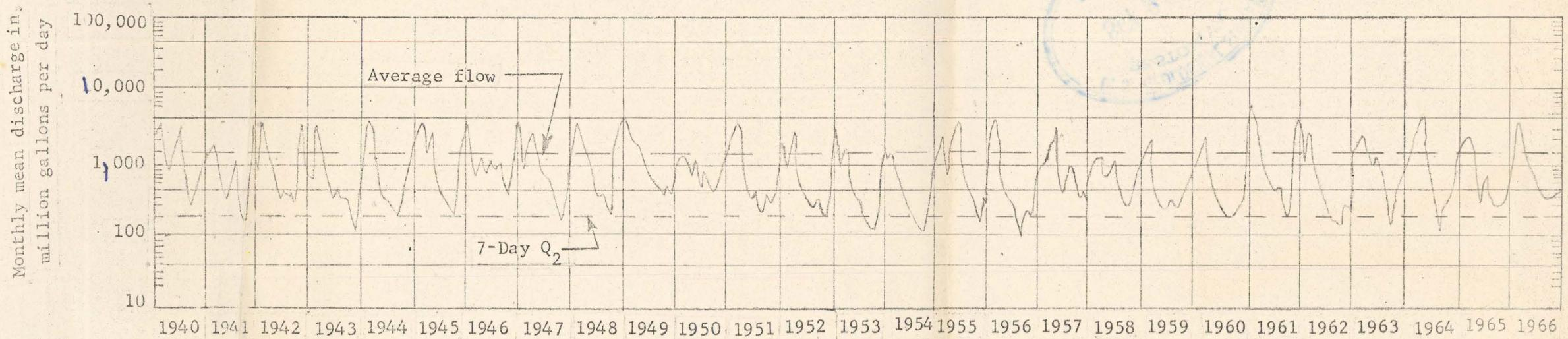
Figure 5.--Hydrograph of mean monthly discharges of Cahaba River at Sprott, Alabama.
