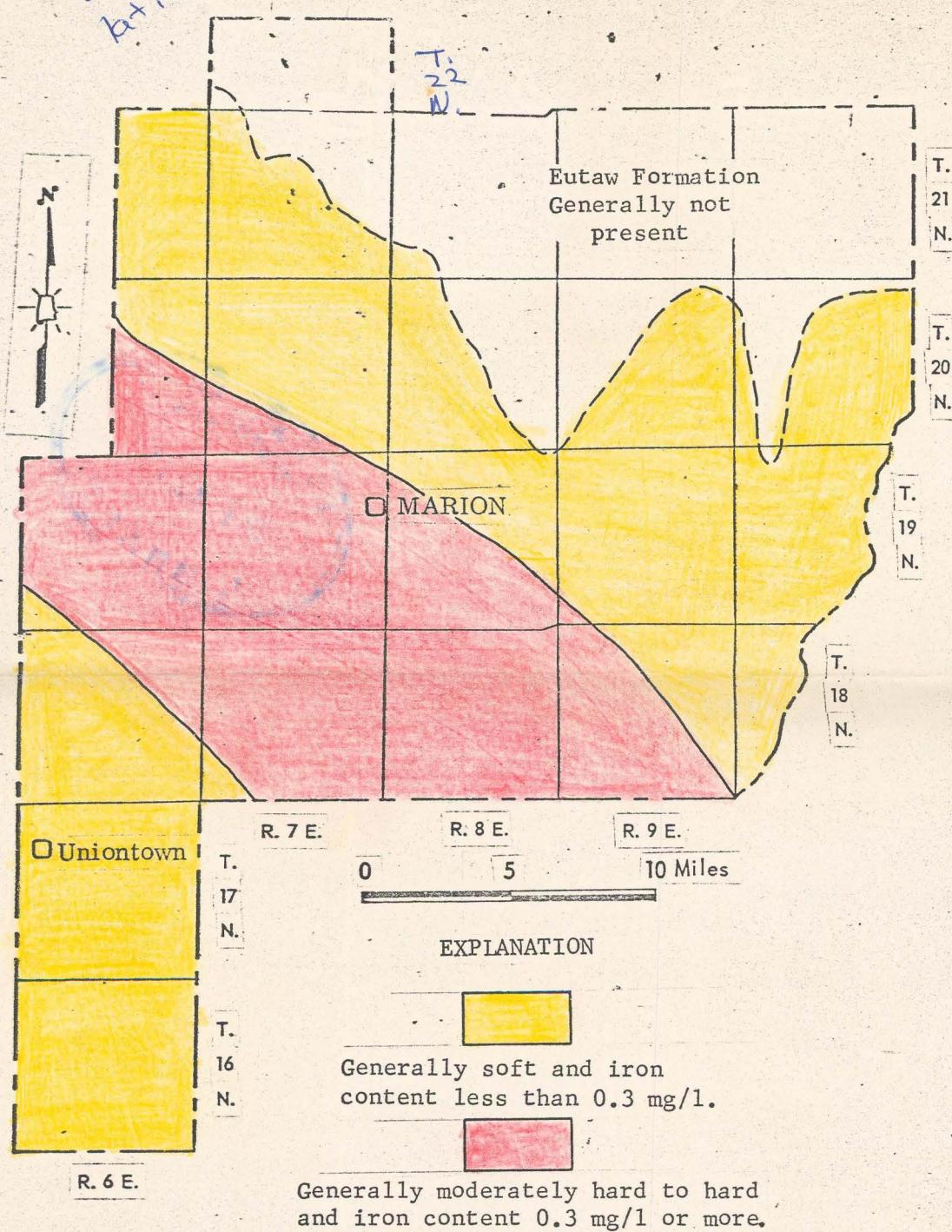
Figure 6.--Distribution of hardness and iron content of water from the Eutaw Formation in Perry County.
