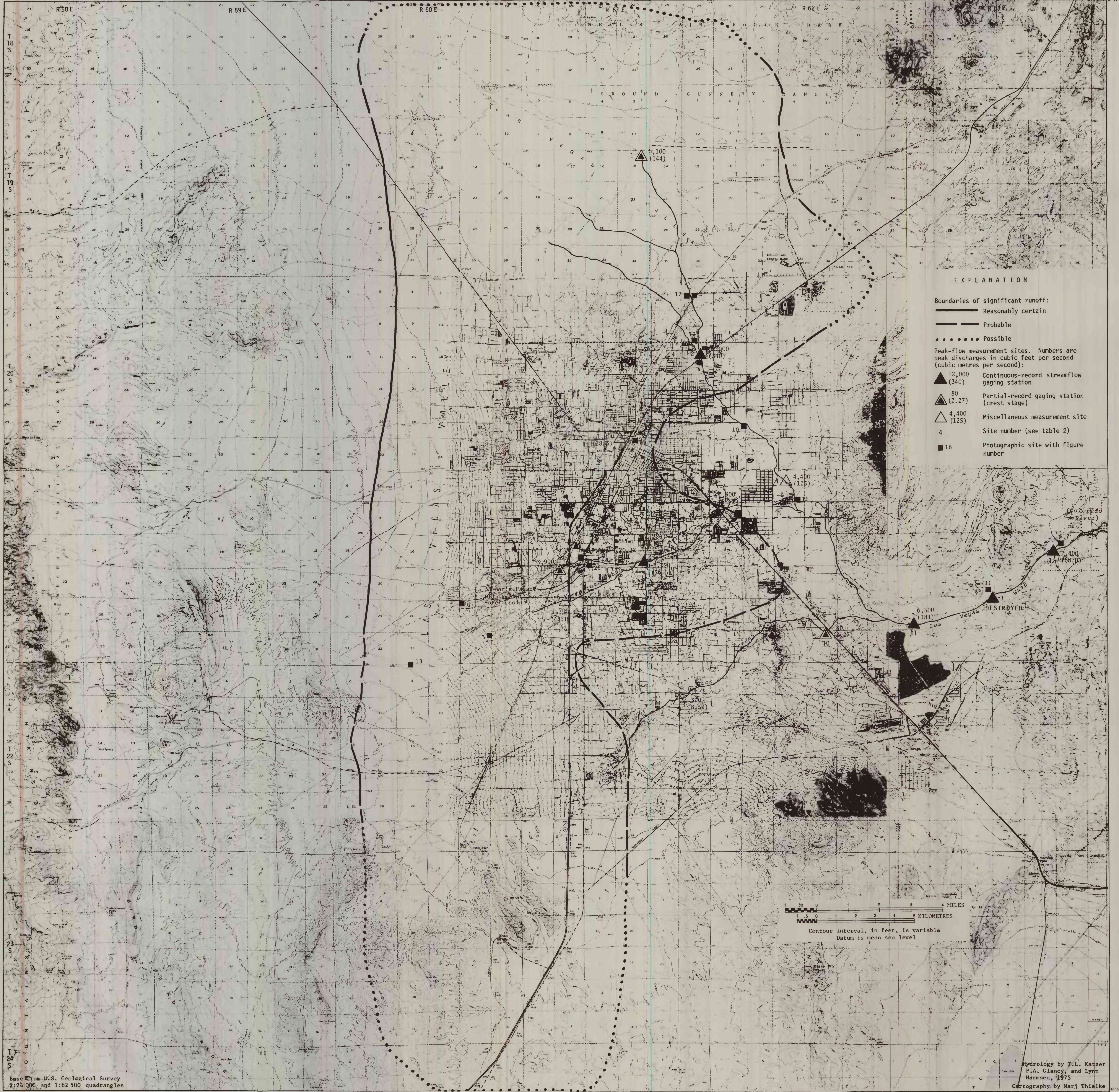
PLATE 1.--MAP OF LAS VEGAS VALLEY, NEVADA, SHOWING EXTENT OF SURFACE-WATER RUNOFF, MEASUREMENT SITES, PEAK DISCHARGES, AND LOCATIONS OF PHOTOGRAPHIC SITES, FOR FLASH FLOOD OF JULY 3-4, 1975.
