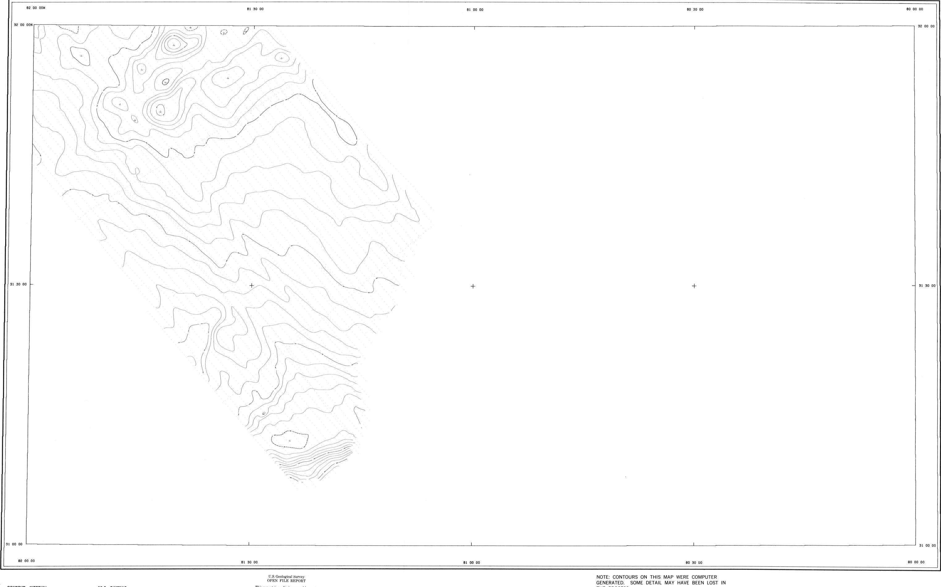
CONTOUR INTERVAL . . . . . . . . . . . . . . . . . 20.0 GAMMAS FLIGHT ALTITUDE ..... 500 FEET AGL INSTRUMENT.... GEOMETRICS G-803 PROTON MAGNETOMETER
