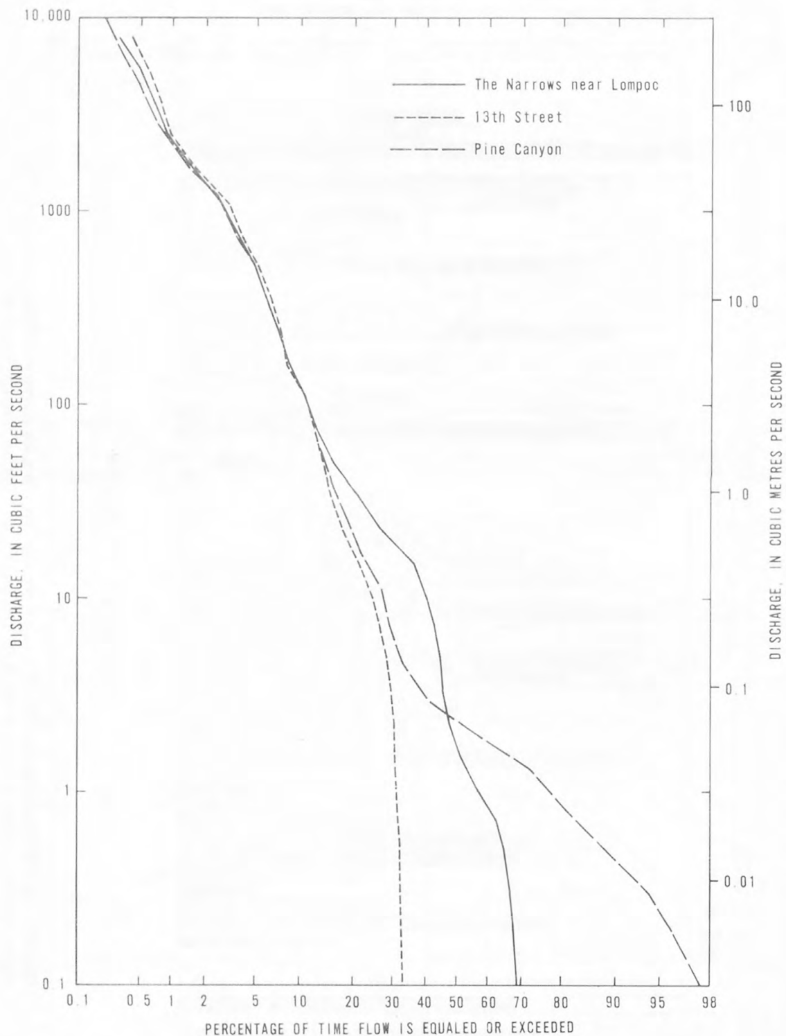
FIGURE 8.--Flow-duration curves at three gaging stations on the Santa Ynez River near Lompoc, water years 1965-71.
