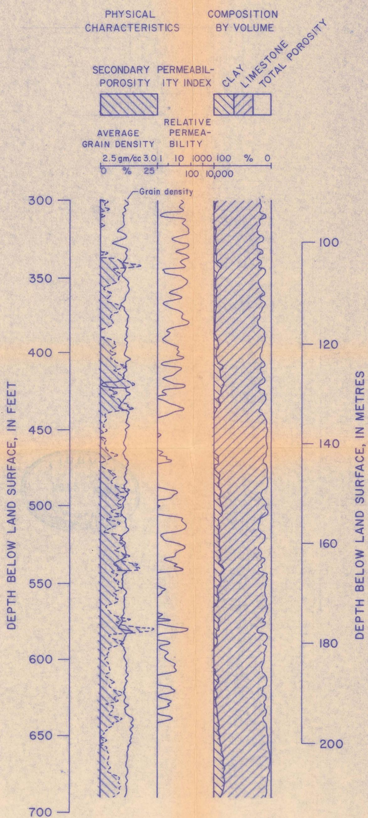
FIGURE 17.-Calculated total porosity, secondary porosity, grain density, permeability, and mineralogy at the Sabinal test hole, YP 69-37-402
