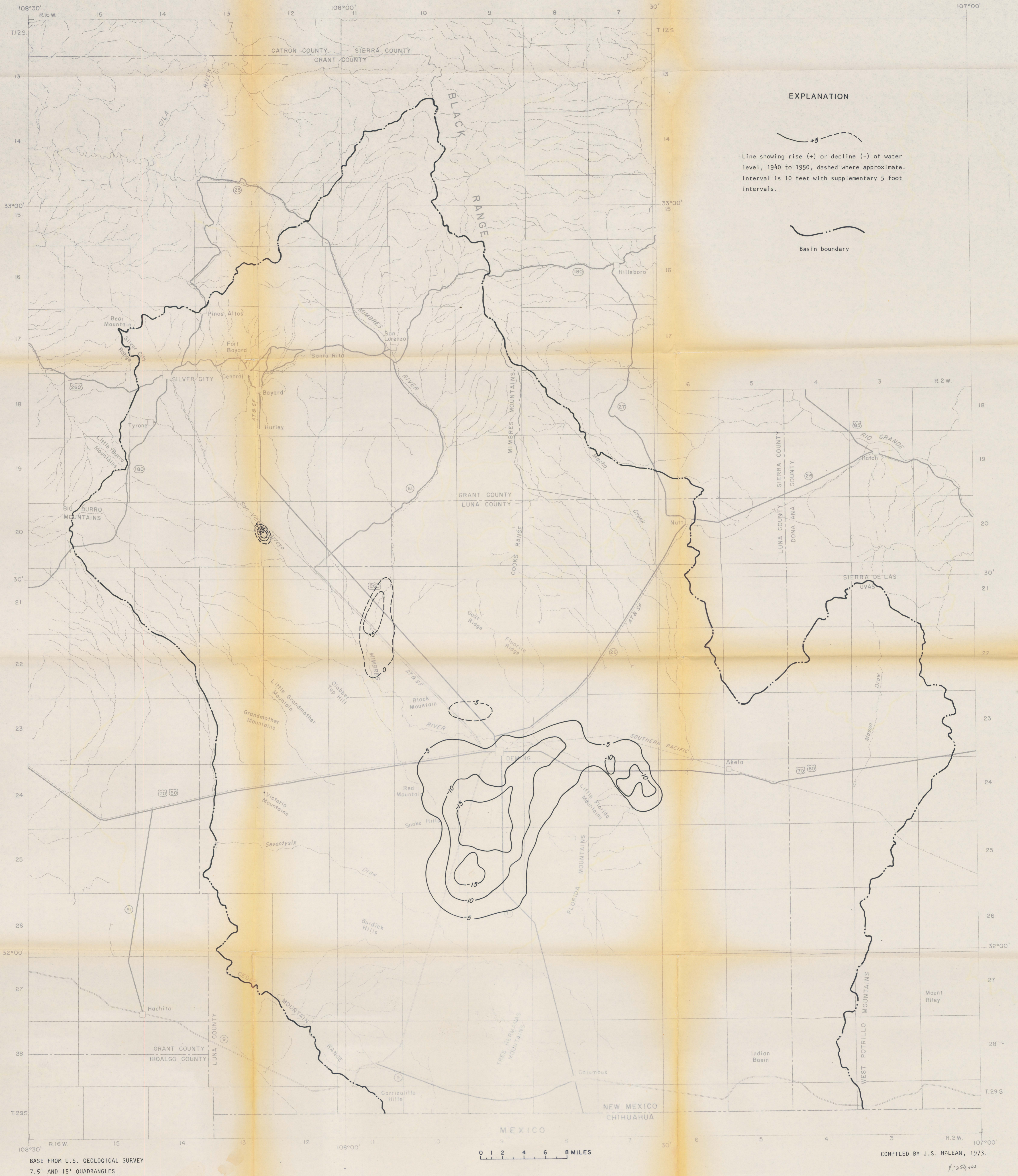
Figure 5.-- Map showing change of ground-water level from 1940 to 1950 in the Mimbres basin, New Mexico.
