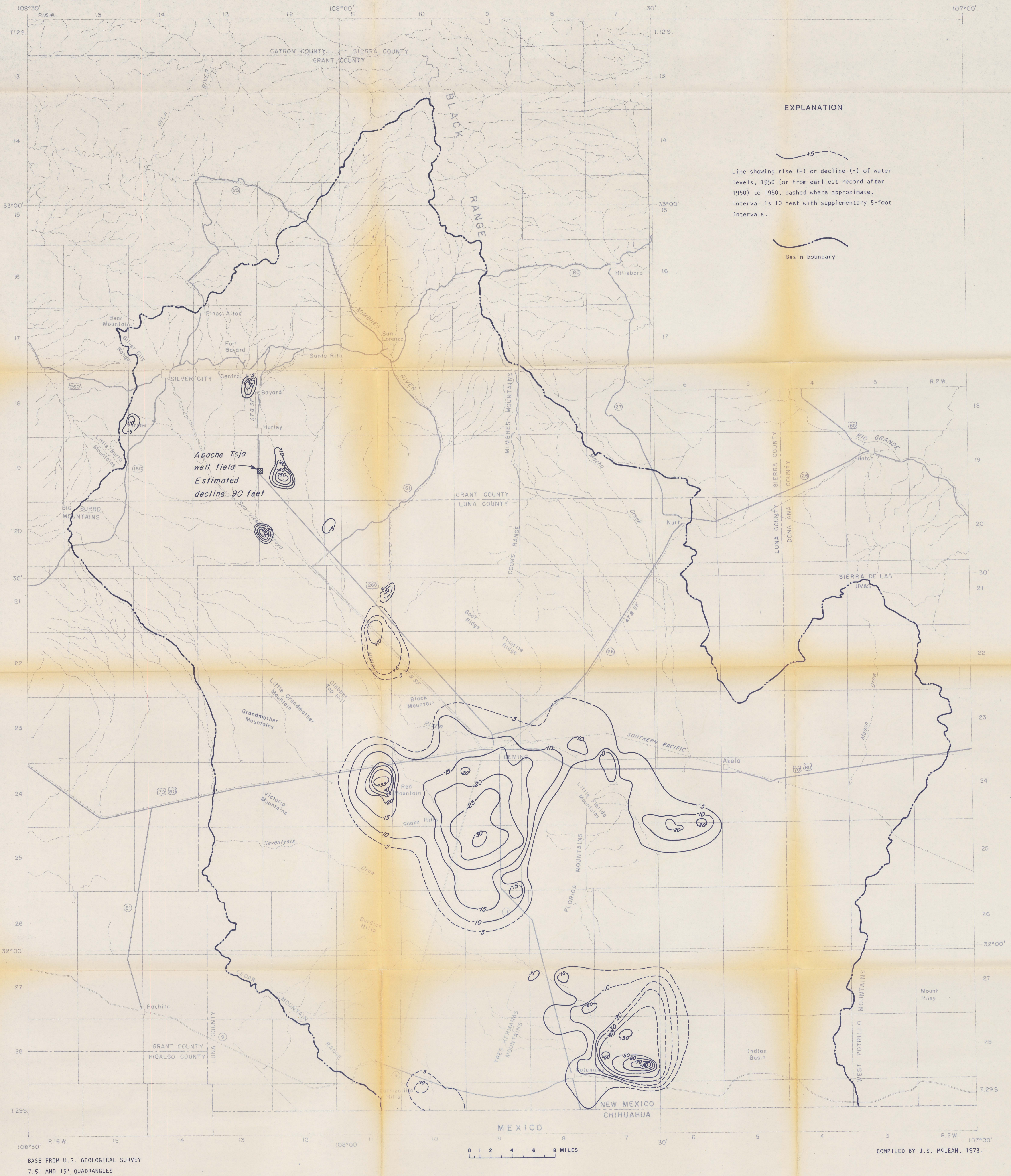
Figure 6.-- Map showing change of ground-water level from 1950-1960 in the Mimbres basin, New Mexico.
