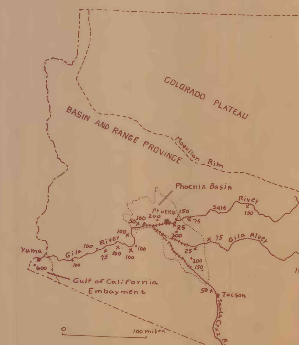
Map showing height of terraces and thickness of flood-plain alluvium in southern Arizona.
