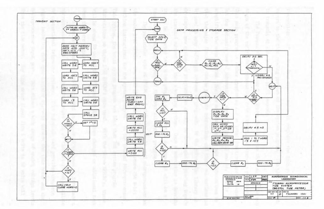
transmitter. After the data transmission is complete the tide system will revert to the tide reading portion of the system program. The time required to transmit 40 tide words is 16.72 seconds.
