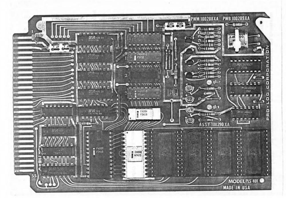
Figure 7. Single Card 4004 Microprocessor System
