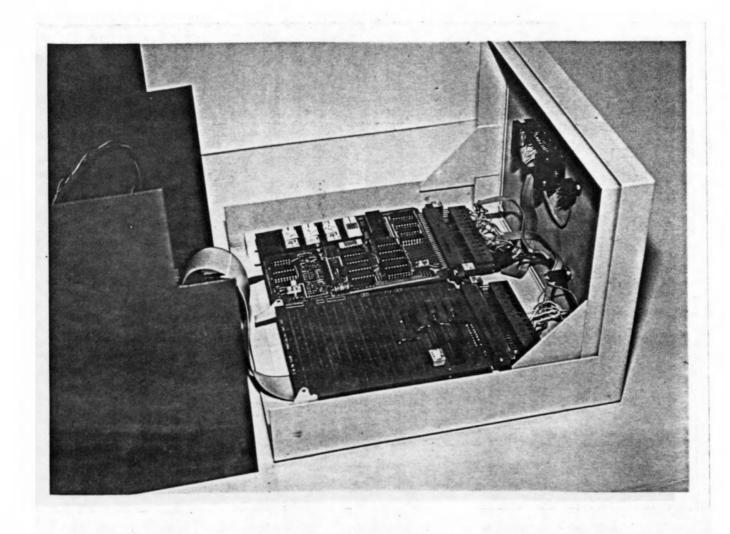
Figure 2. Inside View of Tsunami Microprocessor Tide System
