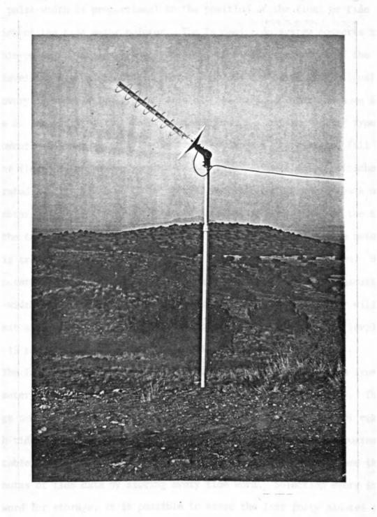
Figure 5. GOES Radio Set Antenna
