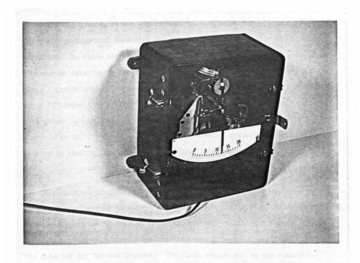
Figure 6. Typical Bristol Float Tide Meter
