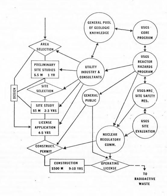
Figure 1. Sources and Flow of Geologic Information During Study, Selection, and Licensing of Reactor Sites and Designs.
