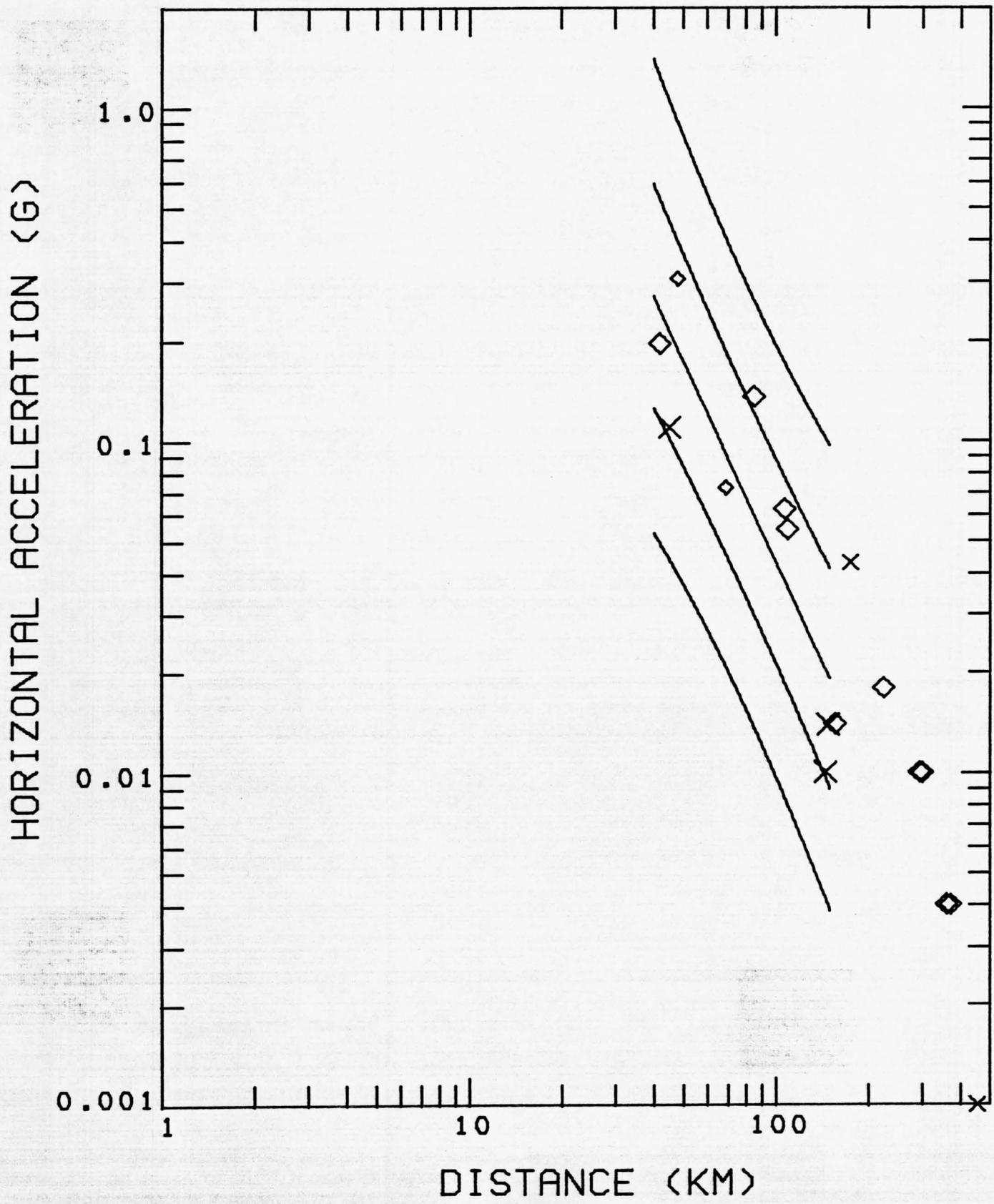
Figure 4. Comparison of the 70 percent prediction intervals for peak horizontal acceleration recorded at the base of small structures for the magnitude classes 5.0-5.7, 6.0-6.4, 7.1-7.7. Curves taken from Figures 1-3.
