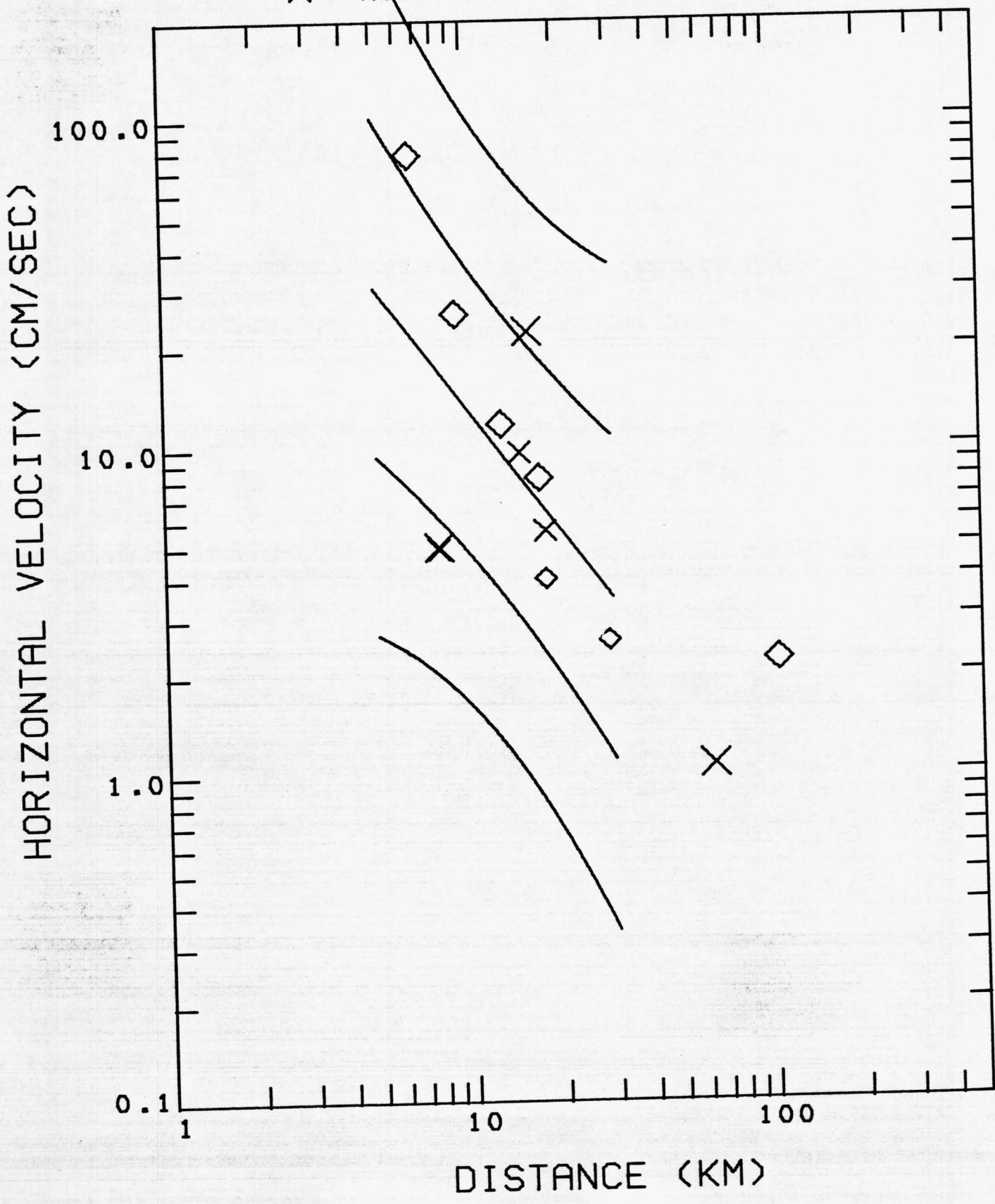
Figure 6. Peak horizontal velocity versus distance to the slipped fault for magnitude 6.4 recorded at the base of small structures. Symbols and curves same as in Figure 1.
