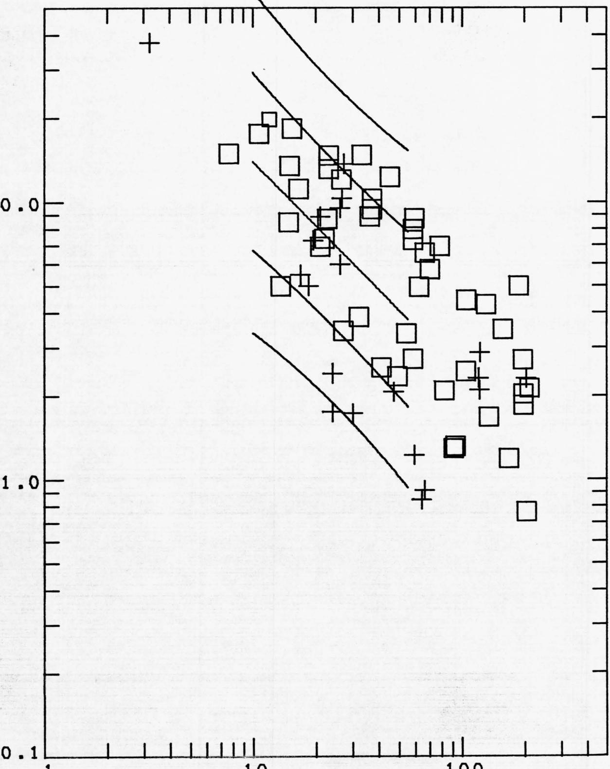
Figure 31. Peak horizontal displacement versus distance to the slipped fault for the magnitude range 7.1-7.7 including data from both large and small structures. Symbols same as in Figure 23.
