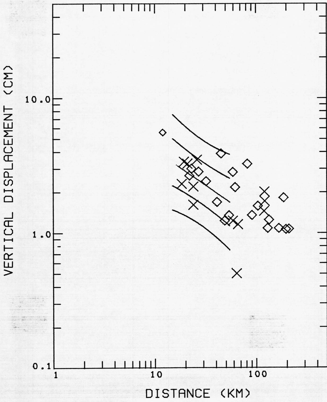
Figure 22. Peak vertical displacement versus distance from the slipped fault for the magnitude range 7.1-7.7 recorded at the base of small structures. Symbols same as in Figure 1.
