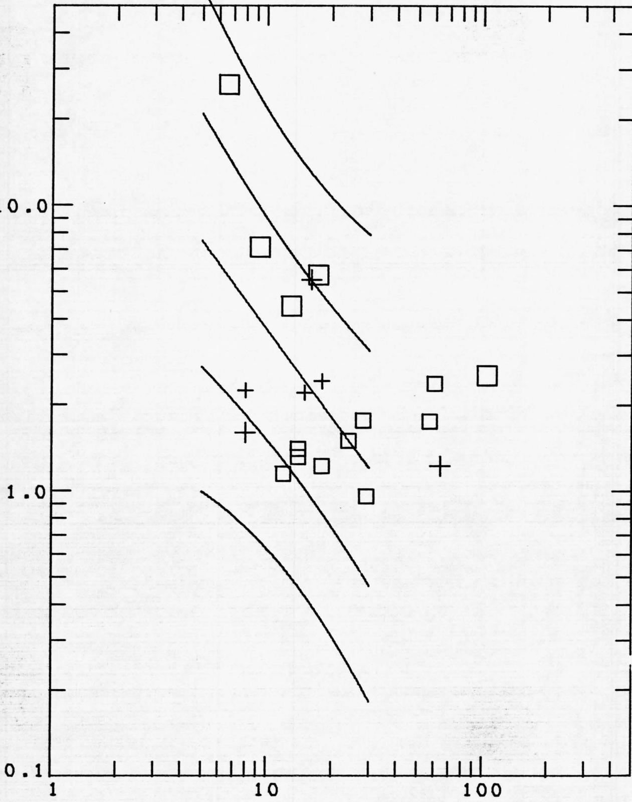
Figure 30. Peak horizontal displacement versus distance to the slipped fault for magnitude 6.4 including data from both large and small structures. Symbols and curves same as in Figure 23.
