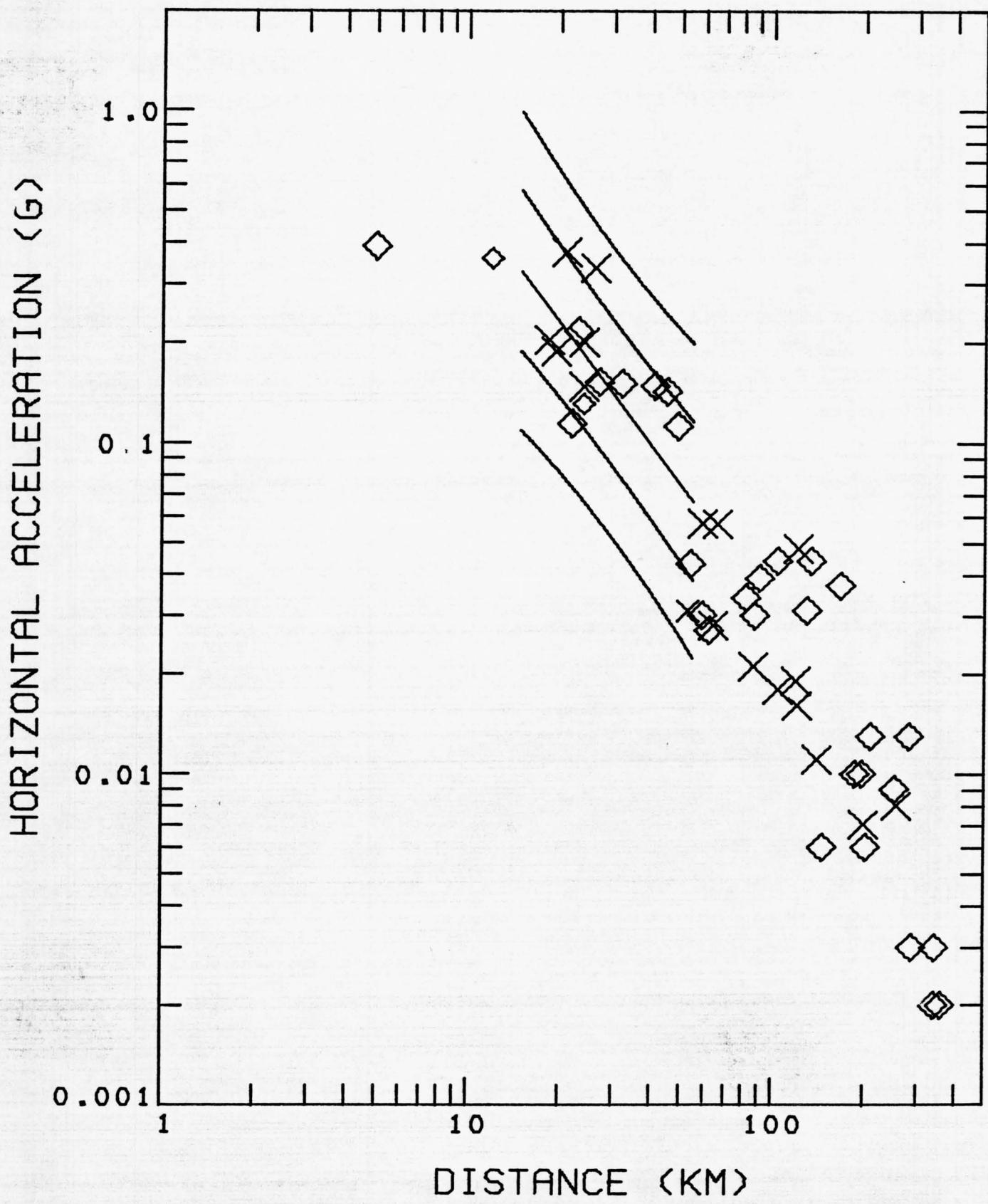
Figure 3. Peak horizontal acceleration versus distance to the slipped fault for the magnitude range 7.1-7.7 recorded at the base of small structures. Symbols and curves same as in Figure 1.
