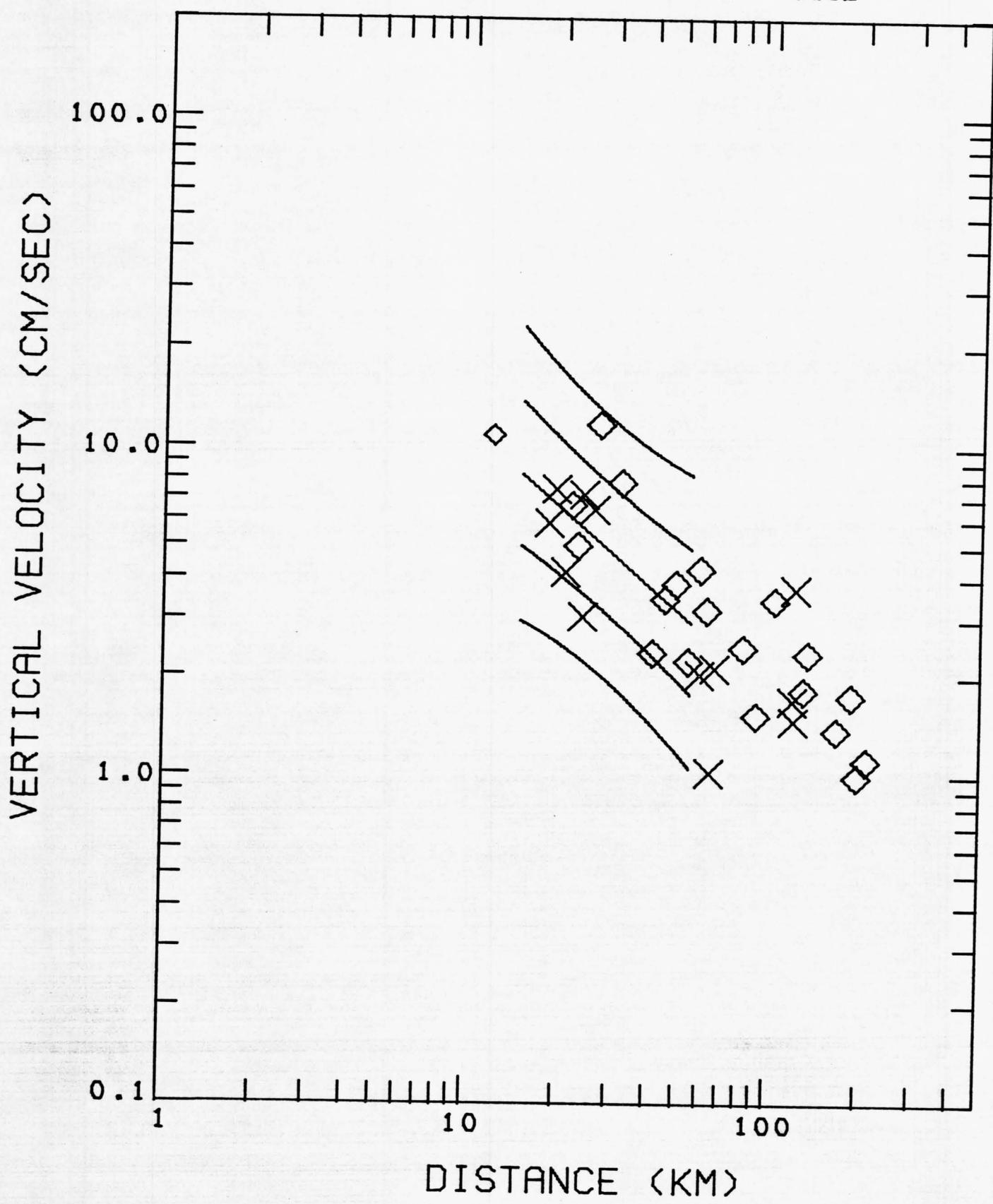
Figure 19. Peak vertical velocity versus distance to the slipped fault for the magnitude range 7.1-7.7 recorded at the base of small structures. Symbols same as in Figure 1.
