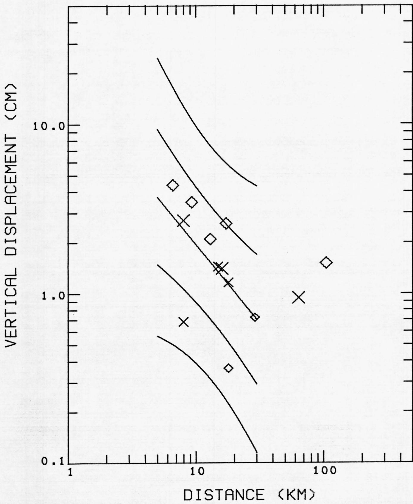
Figure 21. Peak vertical displacement versus distance to the slipped fault
