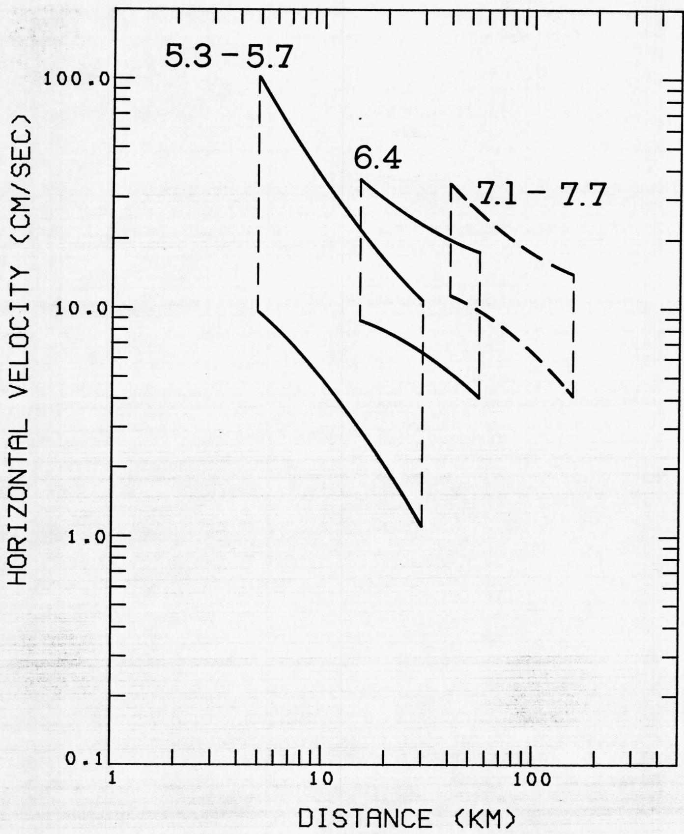
Figure 9. Peak horizontal displacement versus distance to the slipped fault for the magnitude range 5.3-5.7 recorded at the base of small structures. Symbols and curves same as in Figure 1.
