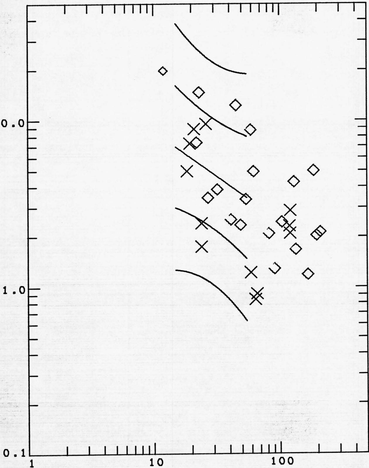
Figure 11. Peak horizontal displacement versus distance to the slipped fault for the magnitude range 7.1-7.7 recorded at the base of small structures. Symbols same as in Figure 1.
