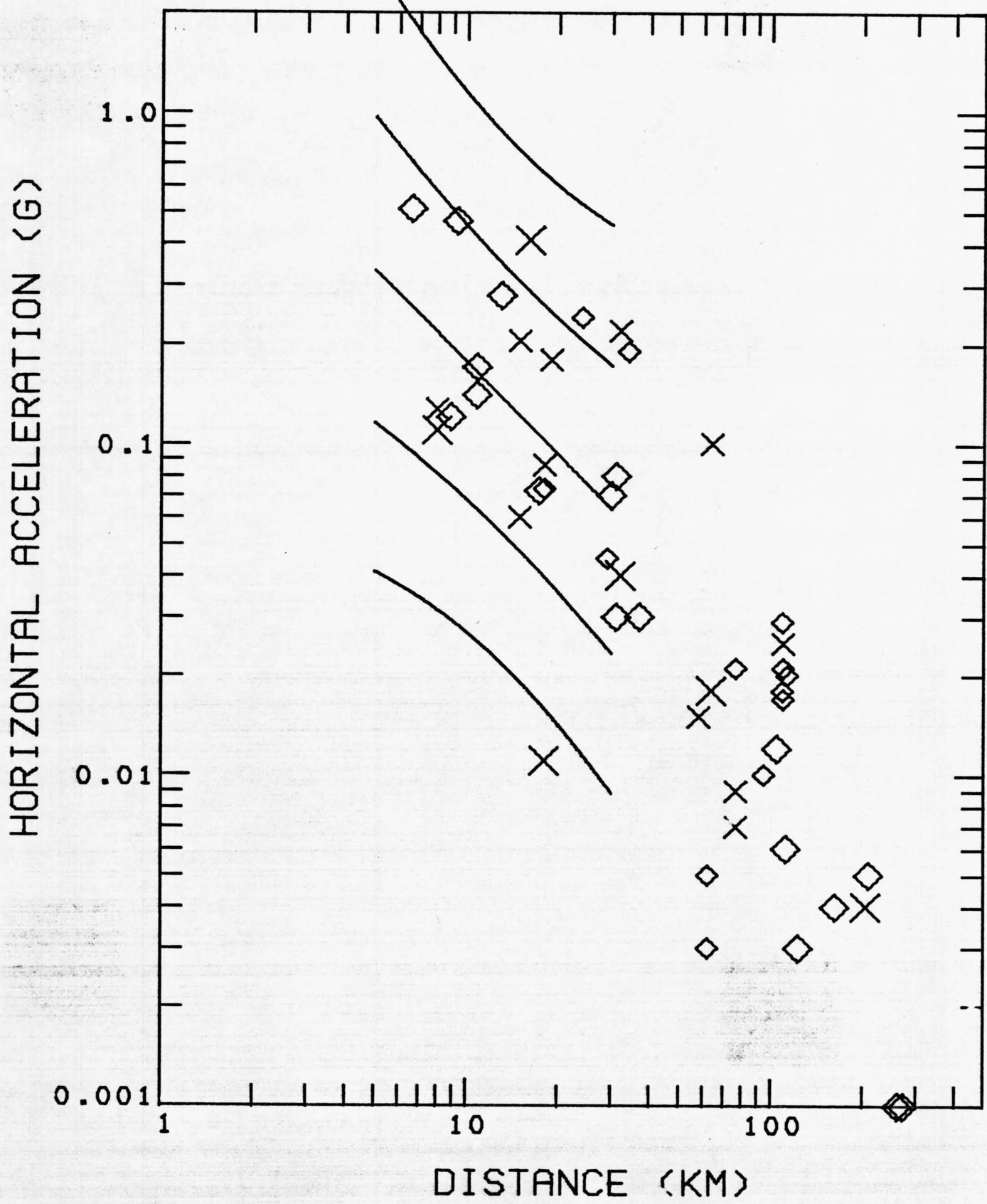
Figure 2. Peak horizontal acceleration versus distance to the slipped fault for the magnitude range 6.0-6.4 recorded at the base of small structures. Symbols and curves same as in Figure 1.
