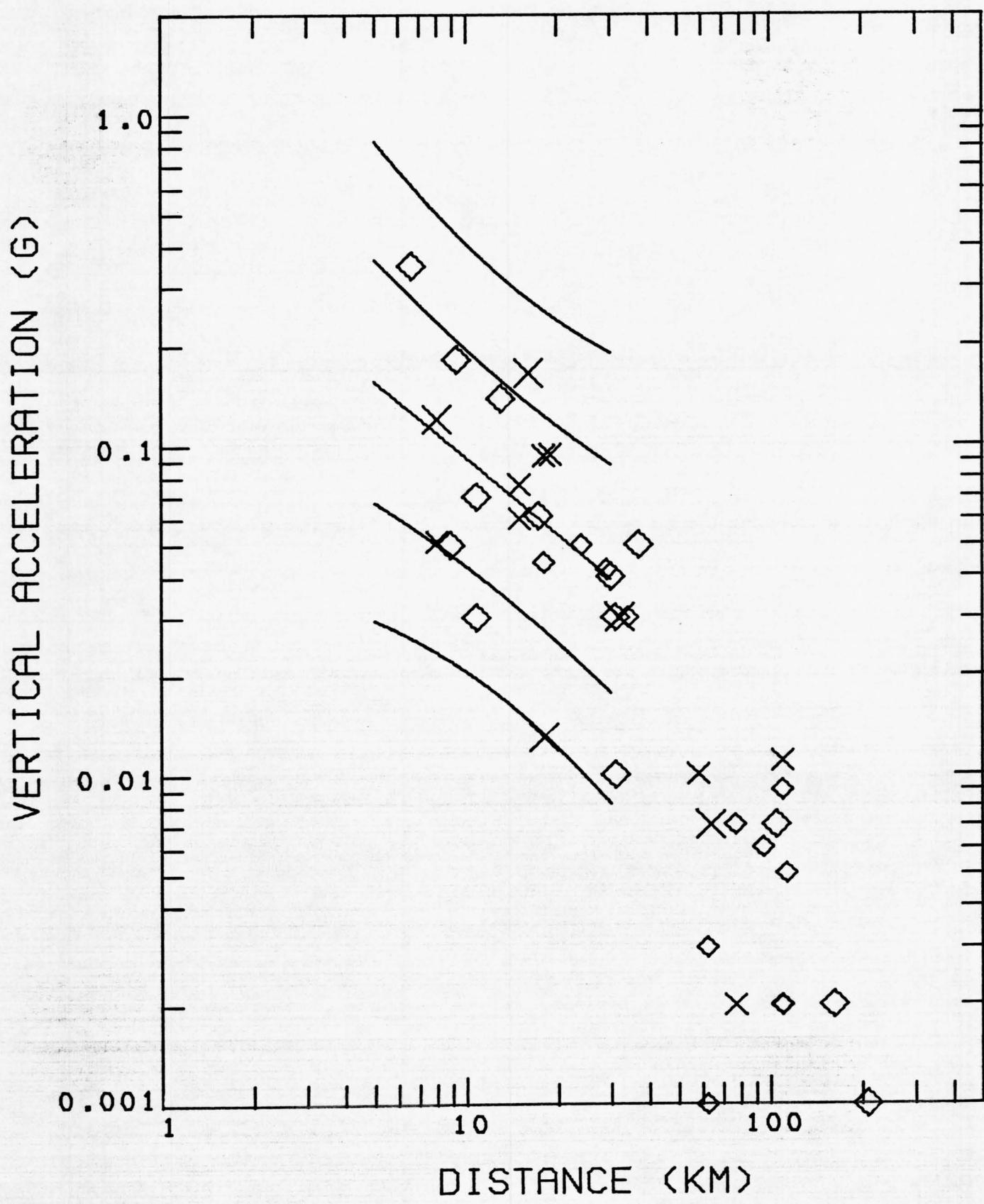
Figure 15. Peak vertical acceleration versus distance to the slipped fault
