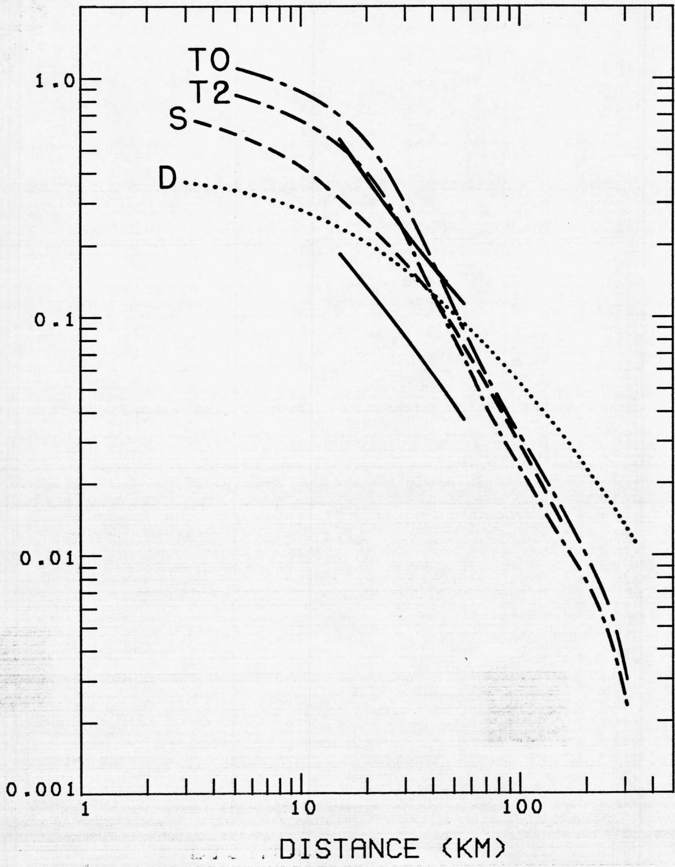
Figure 48. Proposed relationships for peak horizontal acceleration from a magnitude 7.6 earthquake. Curves labeled S, D, T0 and T2 are from the sources given in Figure 41. The solid lines show the 70 percent prediction interval for the small-structure magnitude 7.1-7.7 data set of this report.
