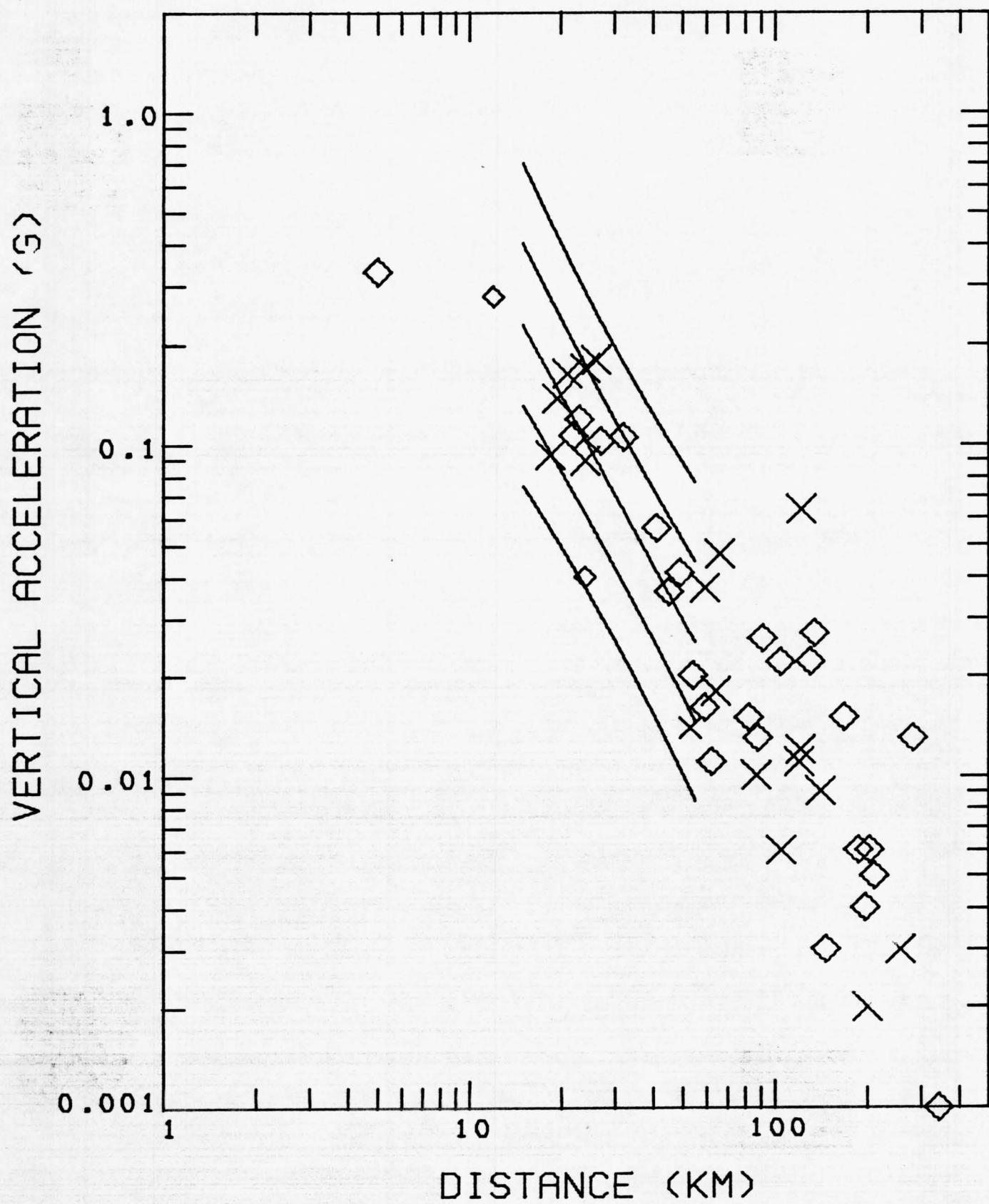
Figure 16. Peak vertical acceleration versus distance to the slipped fault
