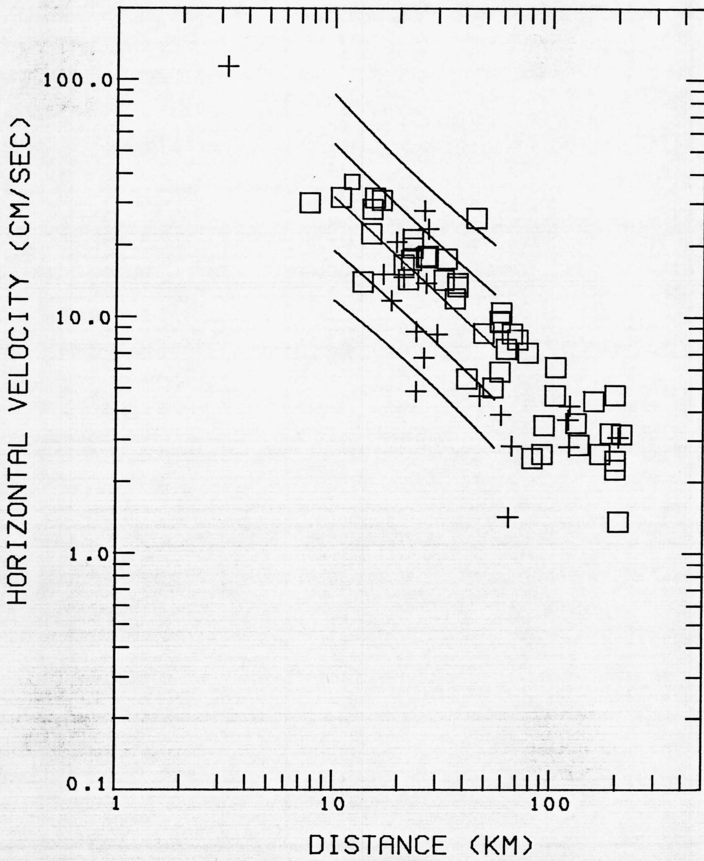
Figure 28. Peak horizontal velocity versus distance to the slipped fault for the magnitude range 7.1-7.7 including data from both large and small structures. Symbols same as in Figure 23.
