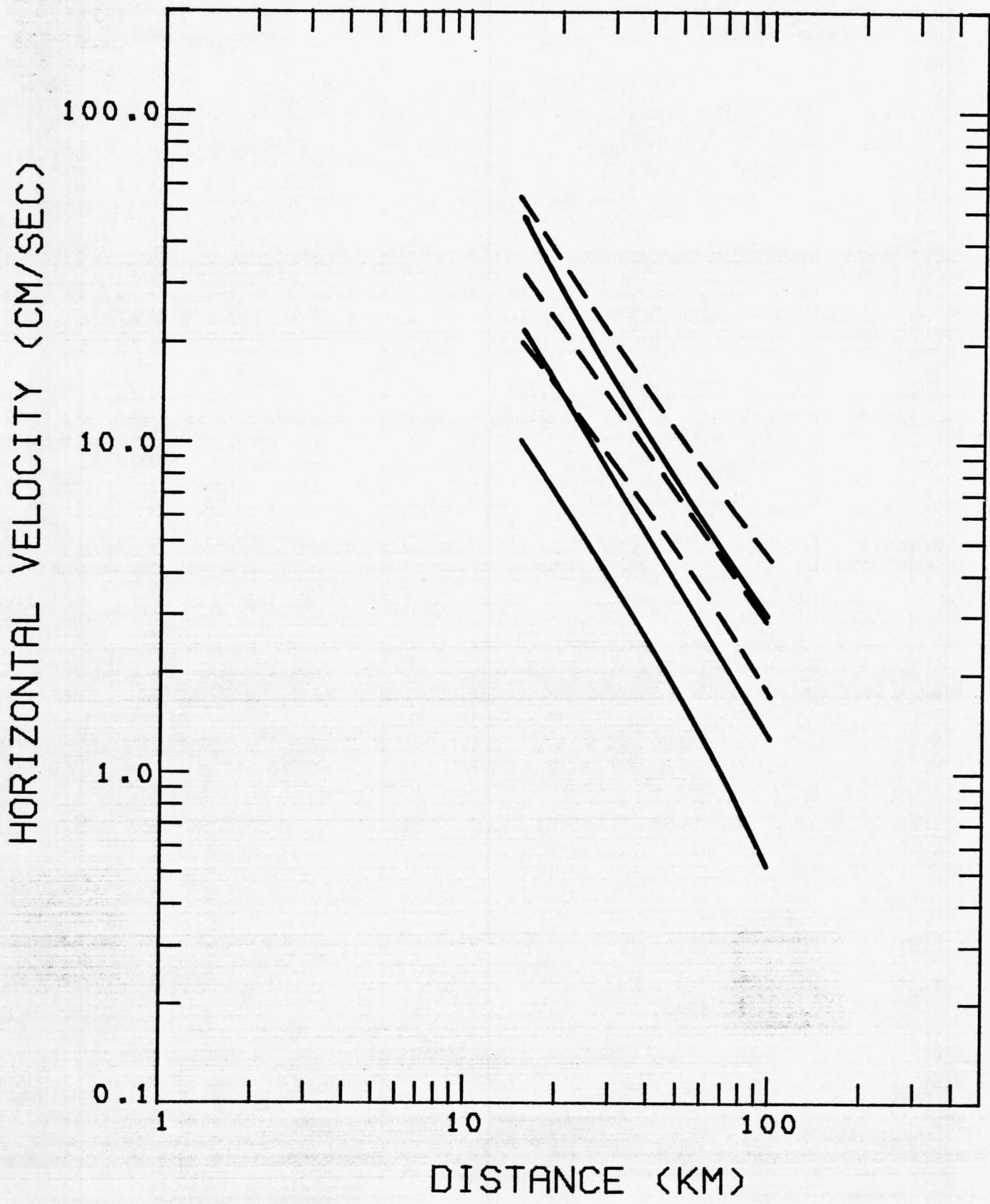
Figure 42. Peak horizontal displacement recorded at the base of small structures versus distance to the slipped fault in the San Fernando earthquake. Symbols same as in Figure 1.
