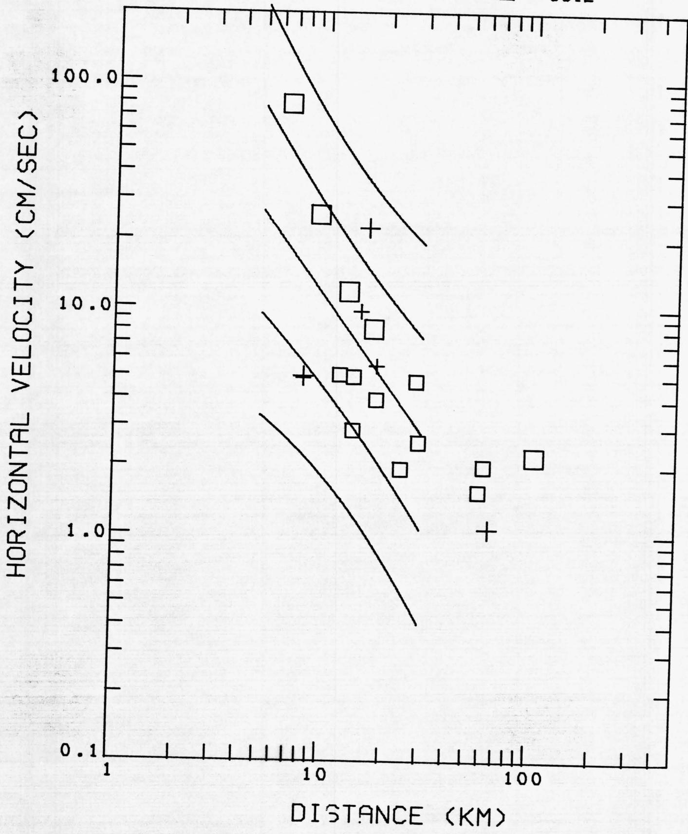
Figure 27. Peak horizontal velocity versus distance to the slipped fault for magnitude 6.4 including data from both large and small structures. Symbols and curves same as in Figure 23.
