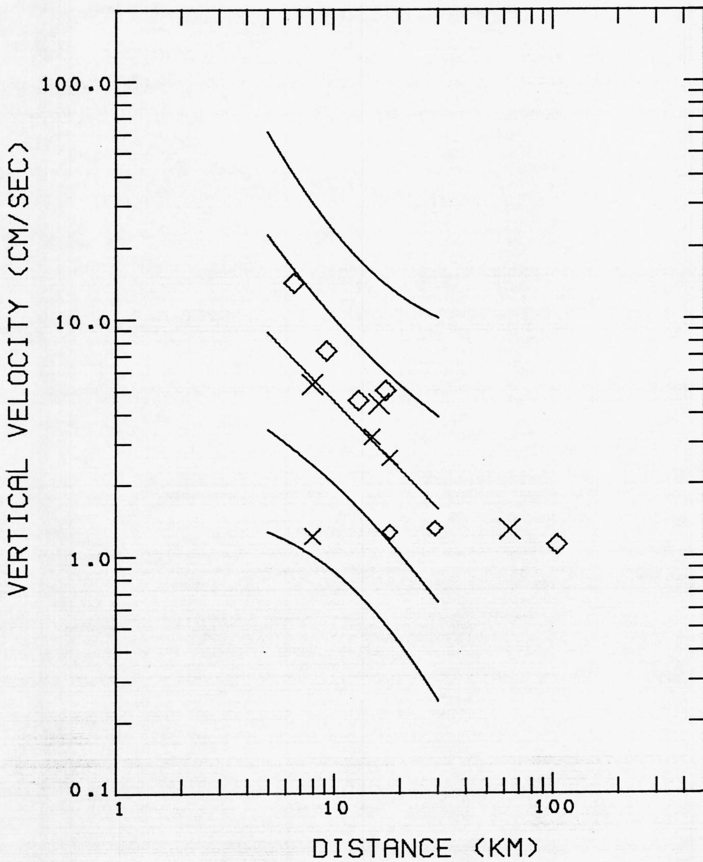
Figure 18. Peak vertical velocity versus distance to the slipped fault for magnitude 6.4 recorded at the base of small structures. Symbols and curves same as in Figure 1.
