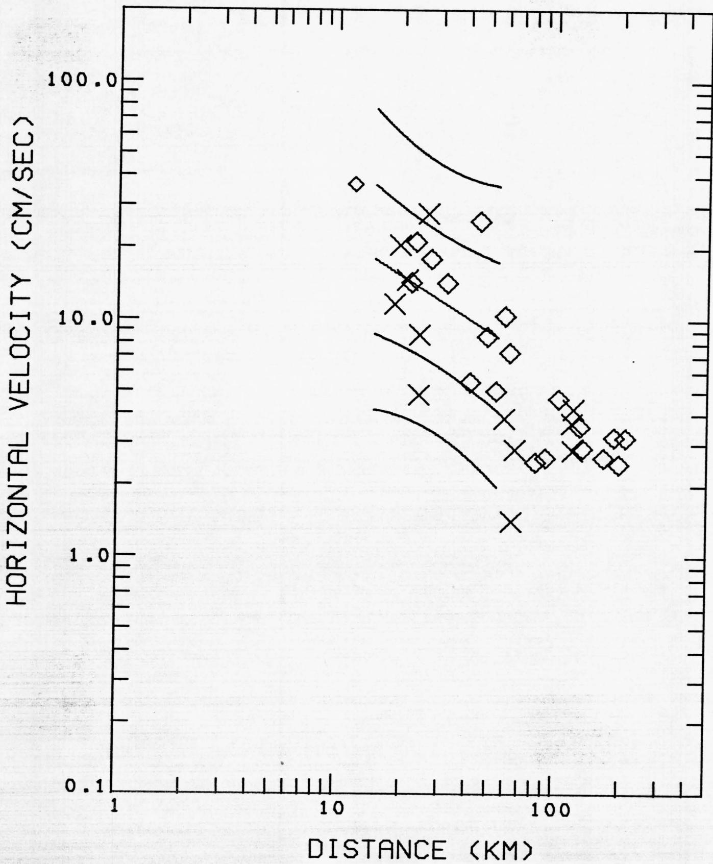
Figure 7. Peak horizontal velocity versus distance to the slipped fault for the magnitude range 7.1-7.7 recorded at the base of small structures. Symbols as in Figure 1.
