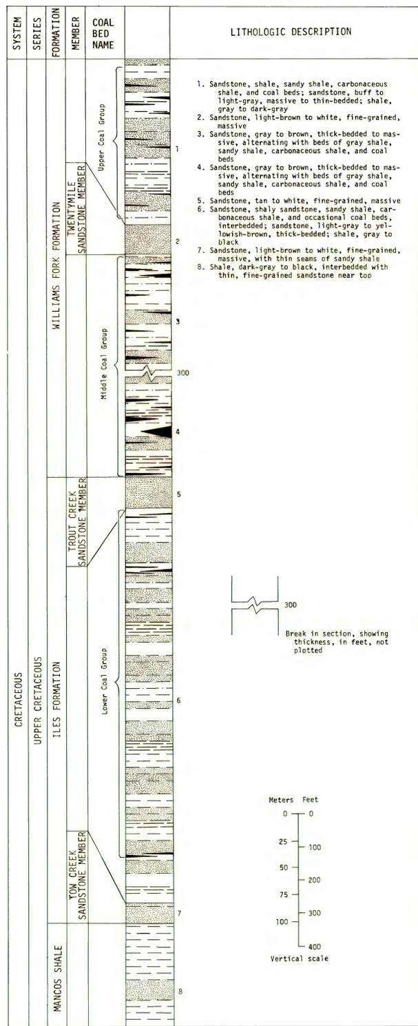
CORRELATION OF COAL BEDS IN DRILL HOLES AND MEASURED SECTIONS
