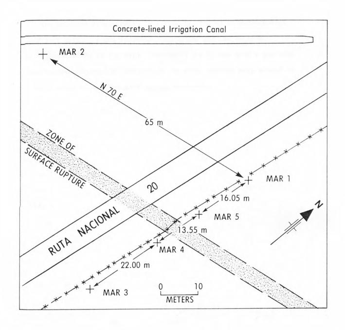
Figure 9. -- Survey station locations for the Marmol alinement array.
