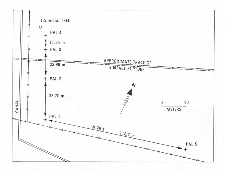
Figure 12. -- Survey station locations for the Palencia array.
