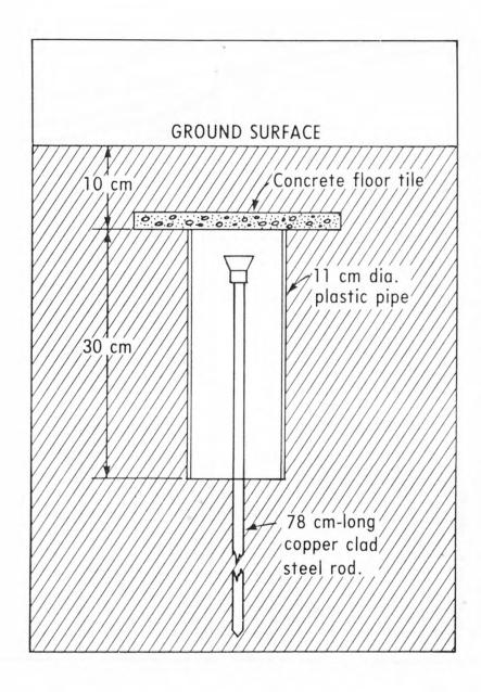
Figure 2.--Cross section showing typical monument installation.
