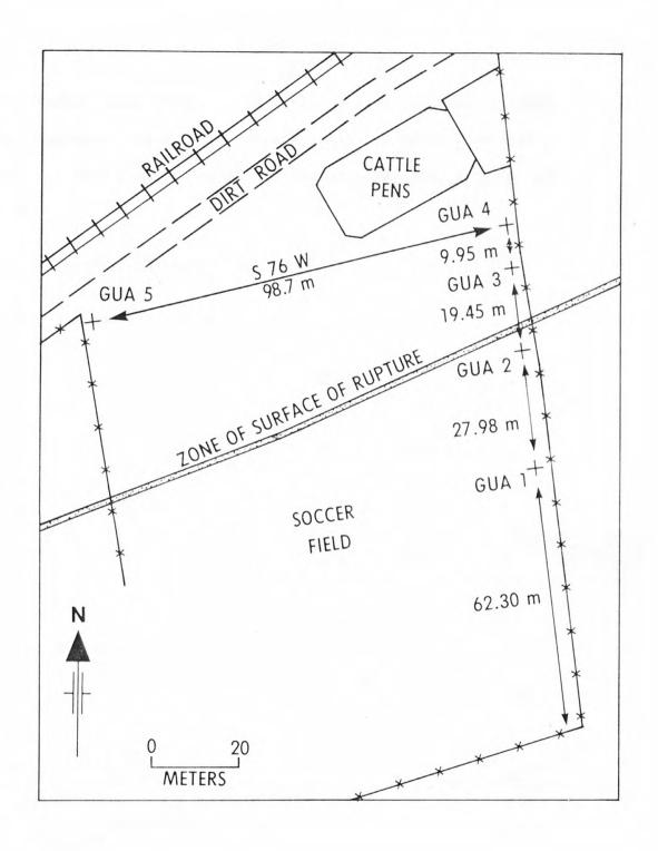
Figure 5.--Survey station locations for the Gualán alinement array.
