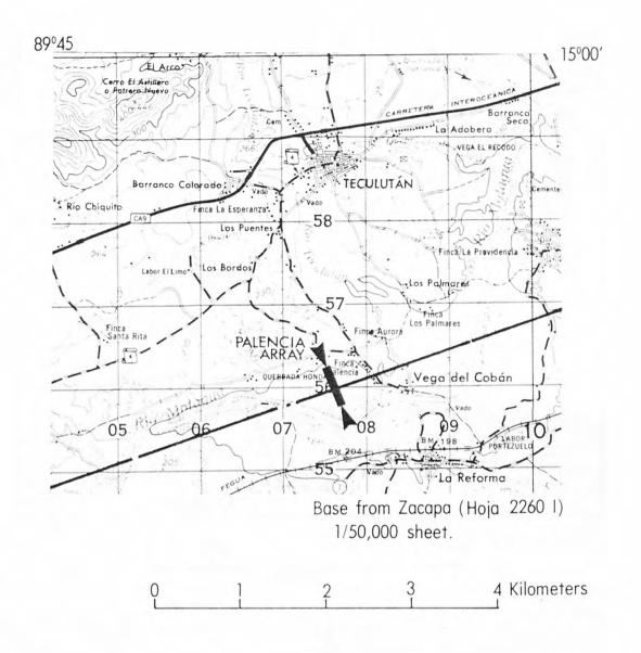
Figure 10.--Location map for the Palencia array. Heavy line shows approximate location of the 4 February 1976 zone of surface faulting.
