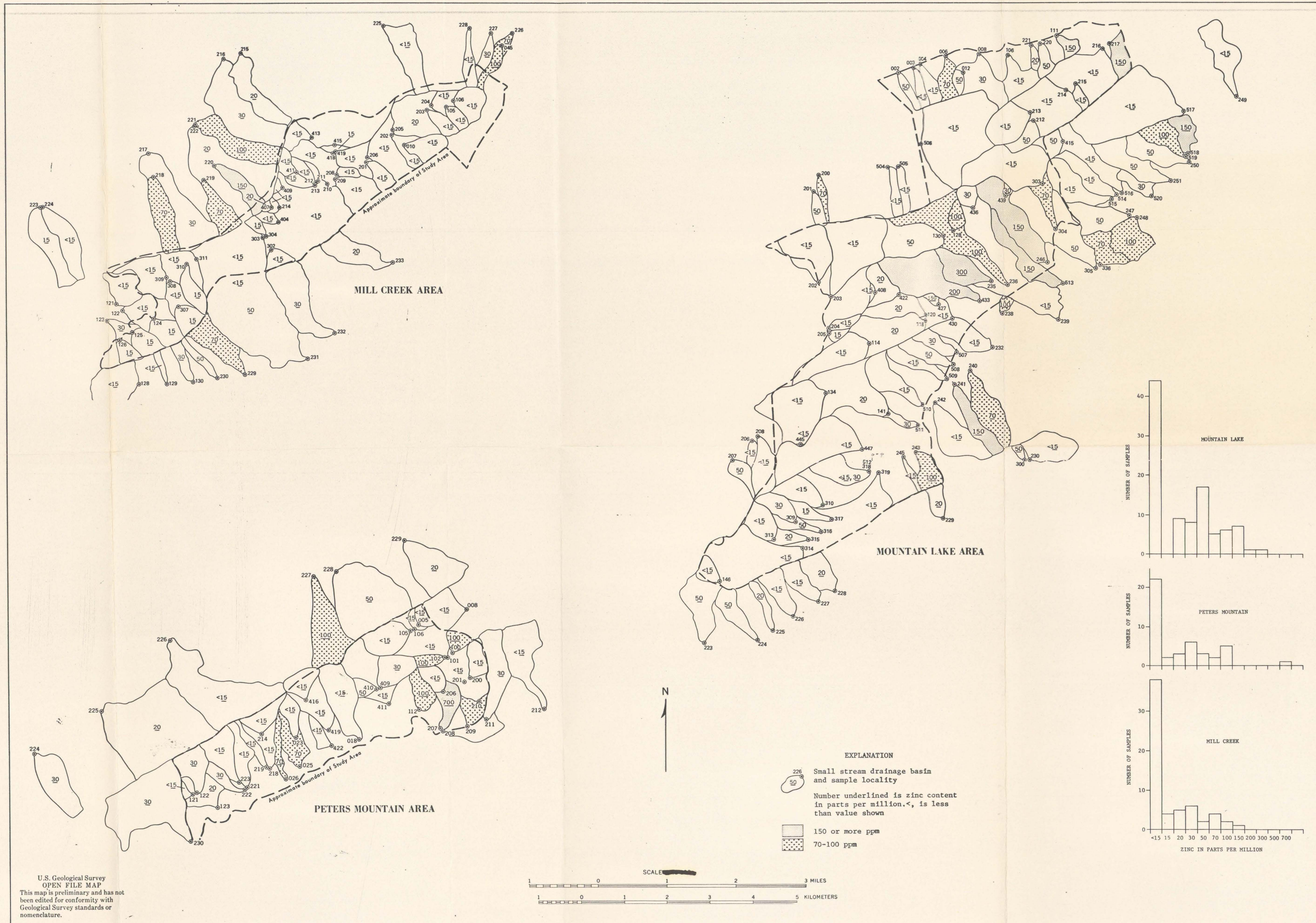
DISTRIBUTION OF ZINC IN STREAM SEDIMENTS IN MILL CREEK, MOUNTAIN LAKE, AND PETERS MOUNTAIN WILDERNESS STUDY AREAS Computerized semiquantitative emission spectrographic data converted to nearest number in the series 1, 1.5, 2, 3, 5, 7, and 10, which represent approximate midpoints of group data on a geometric scale. Original data given in Mei and Lesure (1978), Mei and others (1978), and Rait and Lesure (1978)
