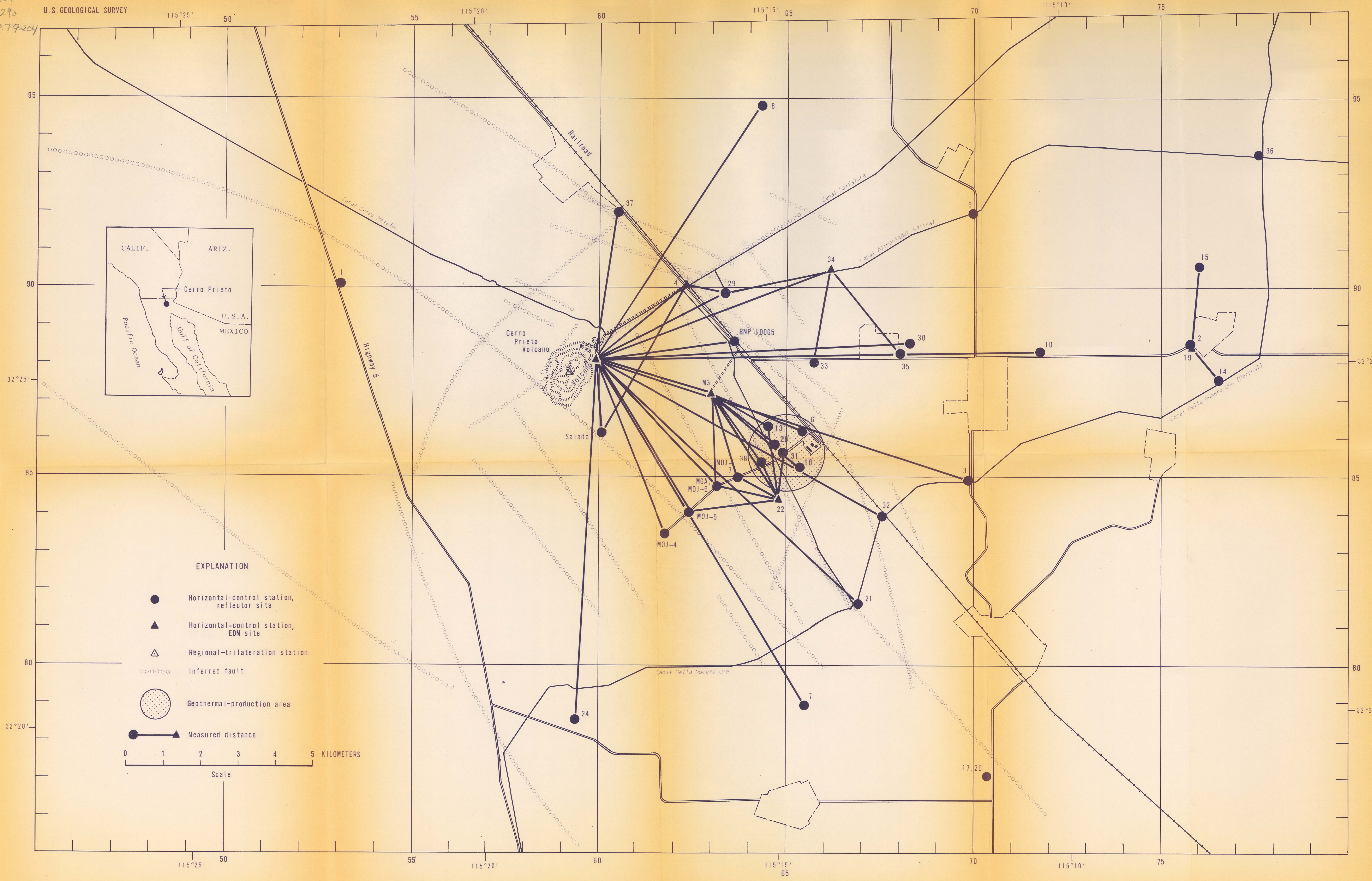
FIGURE 1.—Local network of horizontal-control and inferred faults, Cerro Prieto geothermal area, Mexico.
