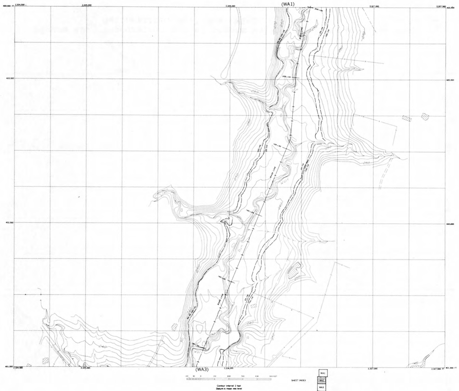
Figure 49. Topographic map of stream valley showing flood boundary delineation, Wolf Run; WA-2
