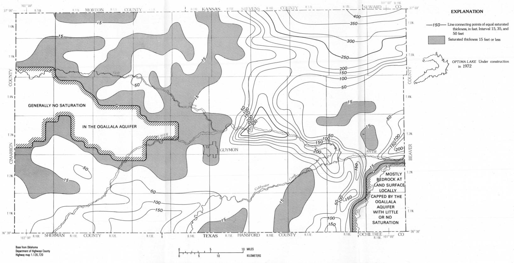
MAP SHOWING SATURATED THICKNESS AT THE END OF MODEL SIMULATION TEST 4, FROM 1972 TO 2013, USING A MINIMUM OF 4 WELLS PER SQUARE MILE AND 1972 PUMPAGE RATE PER WELL, OGALLALA AQUIFER, TEXAS COUNTY, OKLAHOMA.
