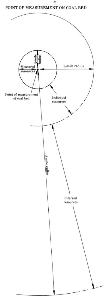
**DIAGRAM SHOWING COMPONENT AREAS OF IDENTIFIED COAL RESOURCES**—Shows arcuate boundary lines enclosing areas of measured, indicated, and inferred coal resources. Boundaries of areas are dashed where projected from an adjacent quadrangle. Areas of measured, indicated, or inferred resources may be present on this map without their outer boundaries being shown. Coal resources beyond the inferred category are hypothetical resources.
