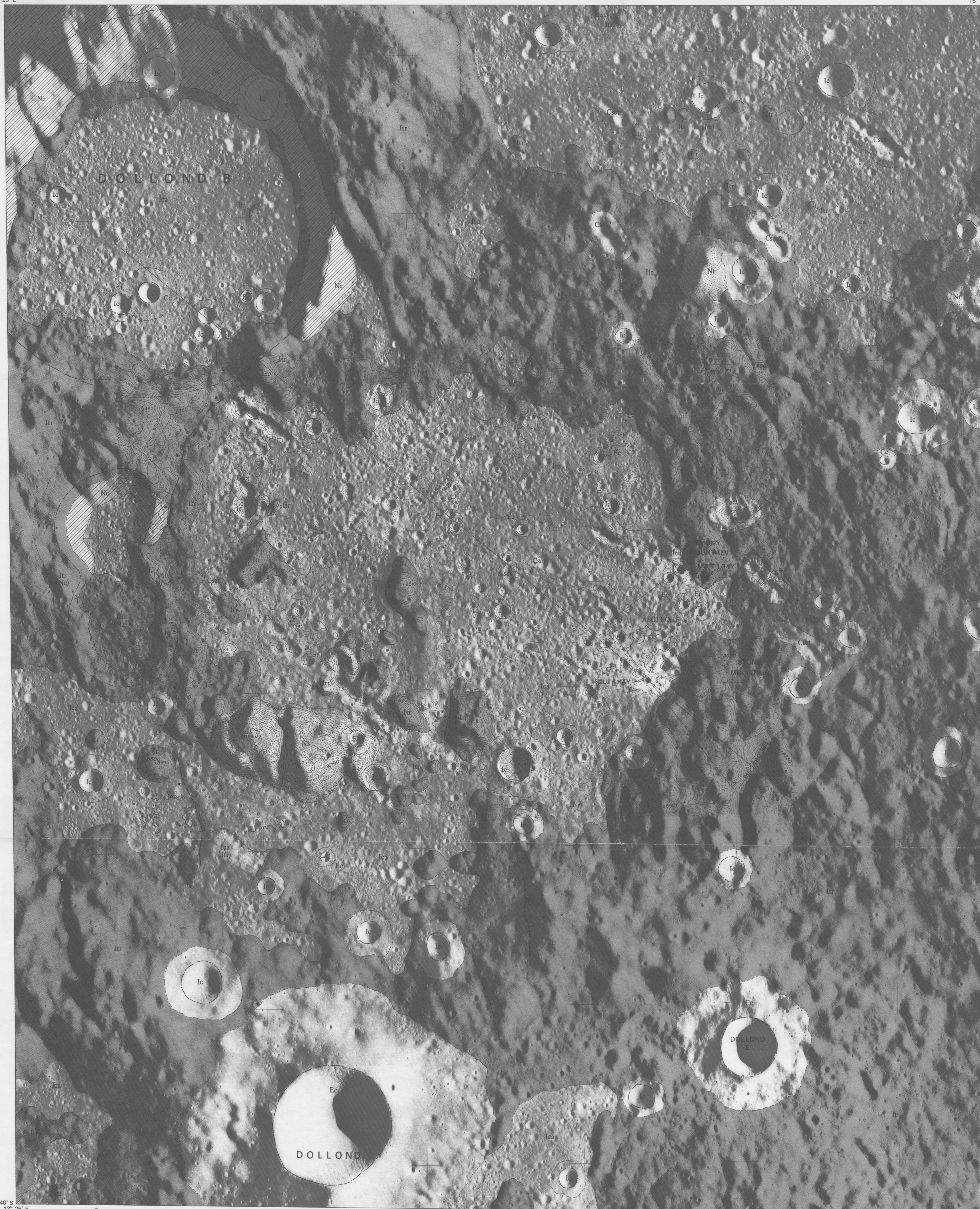
Topographic map of central area compiled at 1:100,000 scale from Apollo 16 metric photographs 975 and 976, on AP/C analytical plotter by Raymond Jordan, U.S. Geological Survey; photographic base from Apollo 16 metric photograph 439. Contours and spot elevations are expressed as radius vectors in meters with the first three digits omitted. For example a radius vector of 1737750 meters is designated as 7750 meters.
