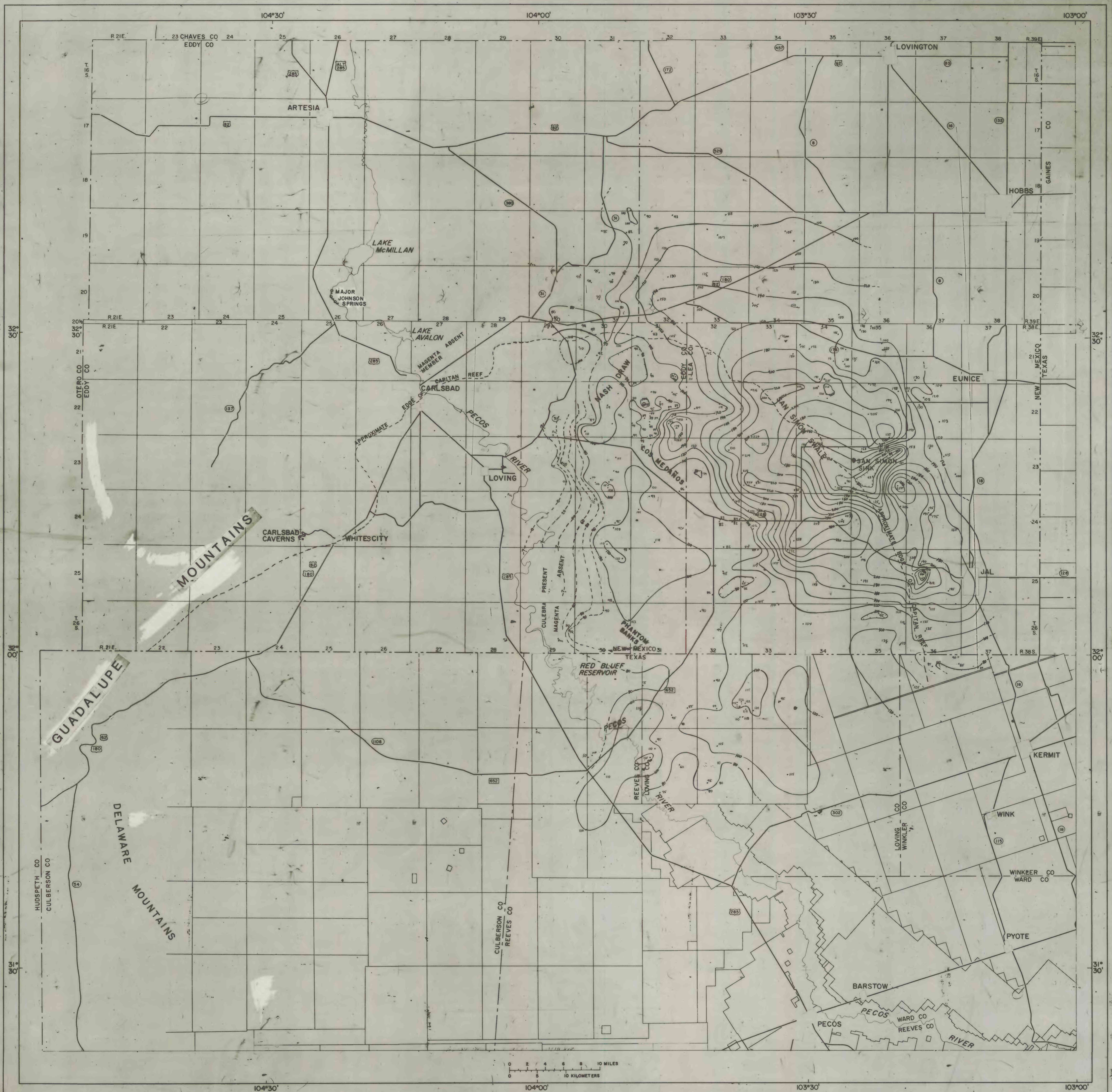
FIGURE 12.--ISOPACH MAP OF THE TAMARISK MEMBER AND THE CULEBRA DOLOMITE MEMBER OF THE RUSTLER FORMATION
