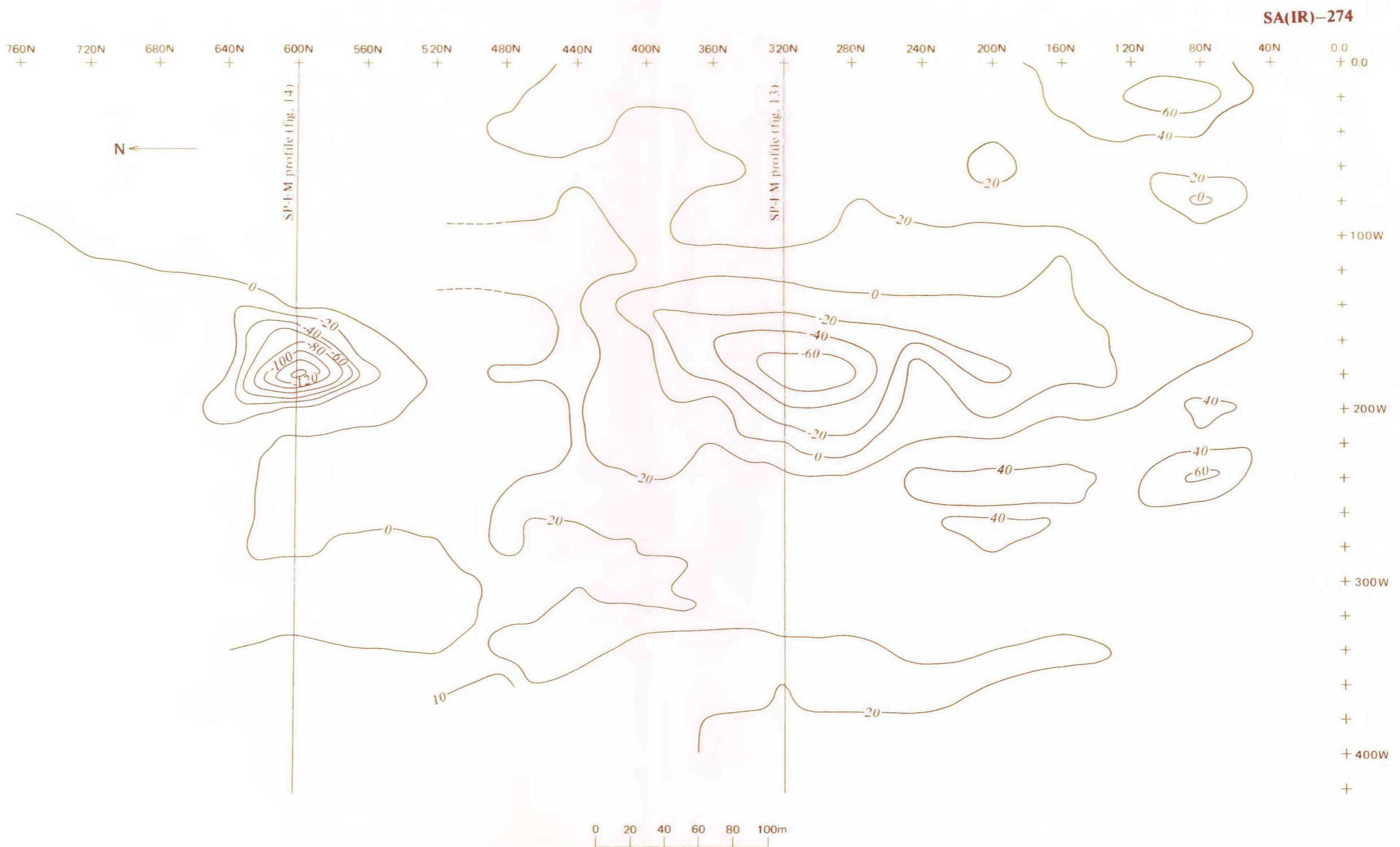
Figure 11.--Self-potential map of Wadi Mandahah ancient mine. Contour interval 20 mv.
