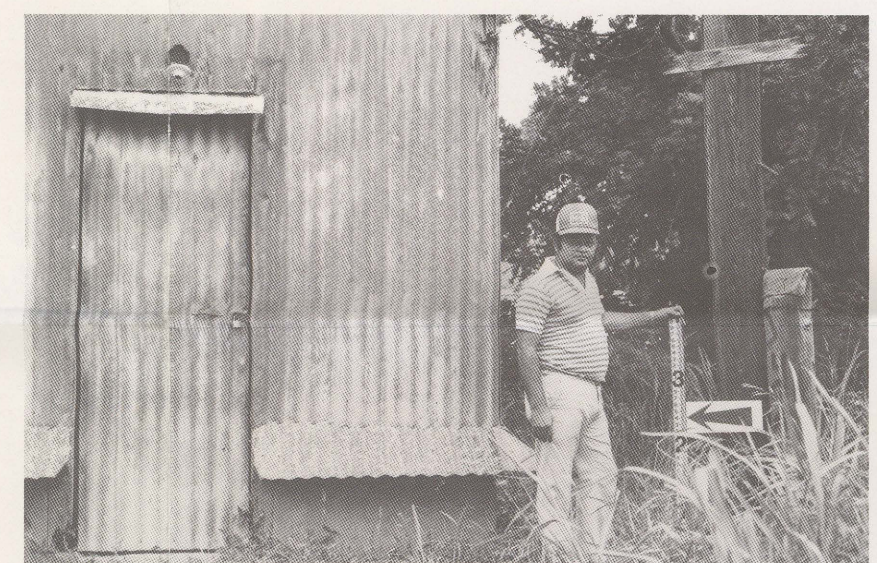
FIGURE 4. - Flood height (noted by arrow) at pump house beside Guayanilla cemetery (photograph B).
