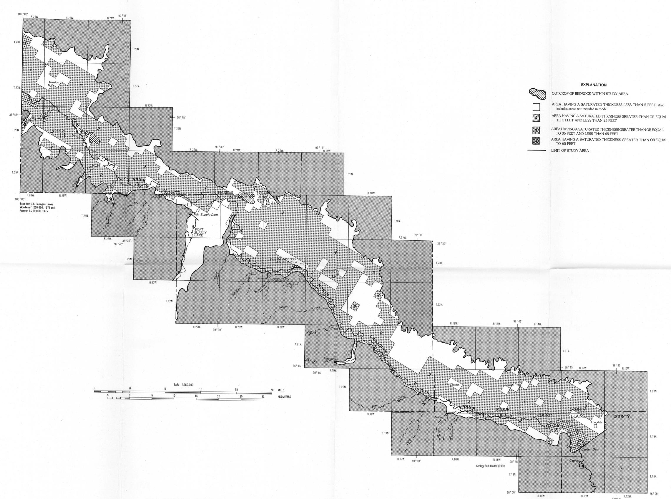
MAP SHOWING SATURATED THICKNESS AT THE END OF MODEL SIMULATION 4 (1993 TO 2020) IN THE ALLUVIUM AND TERRACE AQUIFER ALONG THE BEAVER-NORTH CANADIAN RIVER, NORTHWESTERN OKLAHOMA. THE SIMULATION IS BASED ON A PUMPING RATE OF 1.4 (ACRE-FEET/ACRE)/YEAR OR THE 1977 PUMPING RATE, WHICHEVER IS GREATER, FOR ALL AREAS HAVING 5 FEET OR MORE SATURATED THICKNESS.
